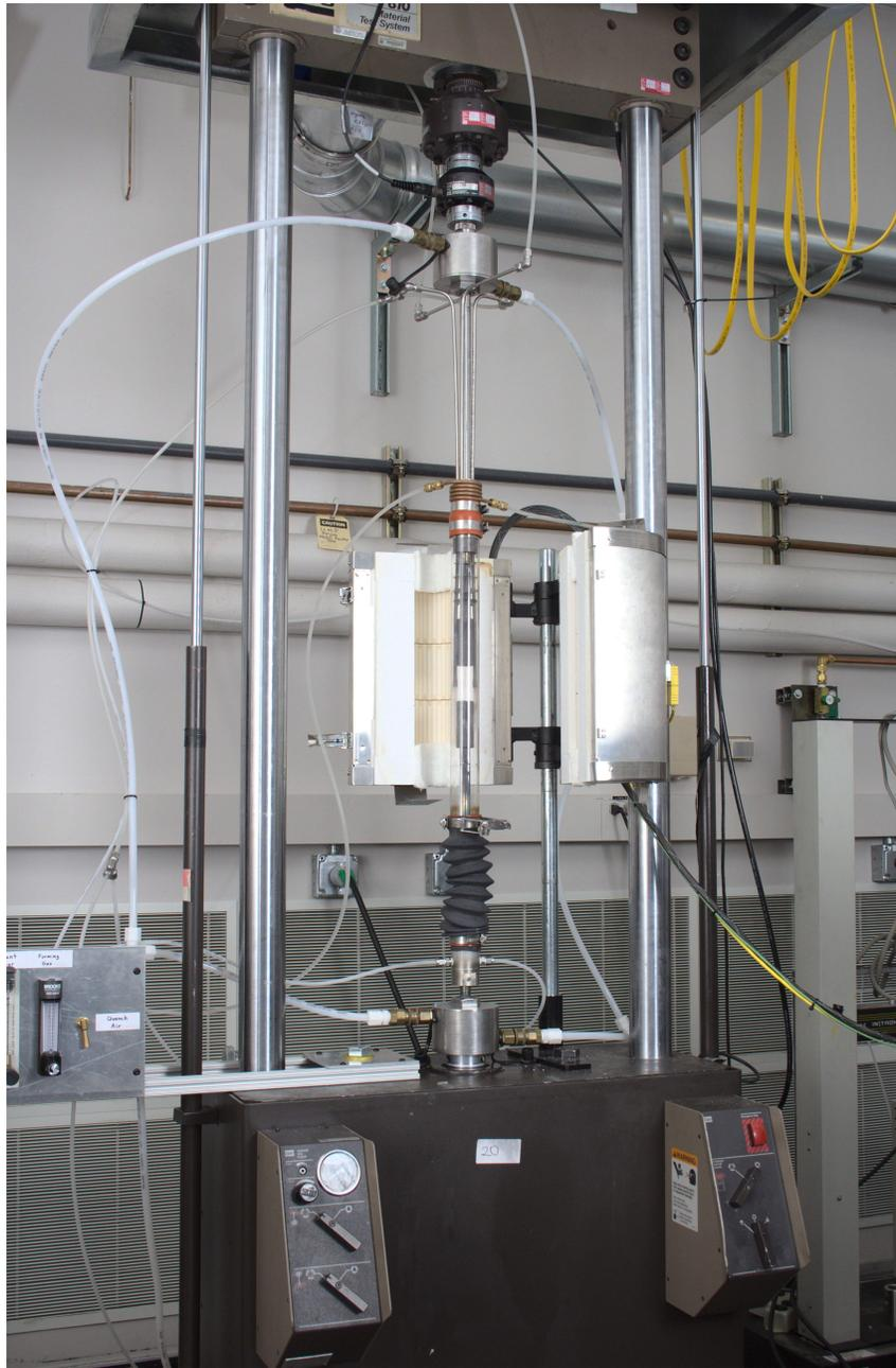
Figure 2.8: This photograph shows the completed assembly of the tensile fixture attached to the MTS 810 test frame.
