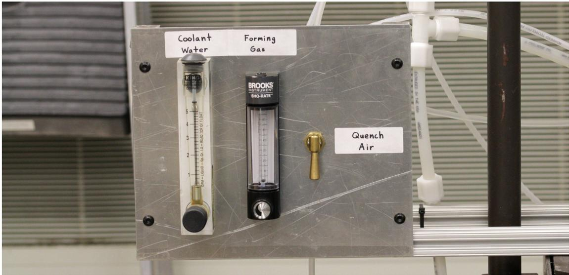
Figure 2.7: This photograph shows the flow control panel for the cooling water, forming gas, and quench air attached to the MTS 810 test frame.
