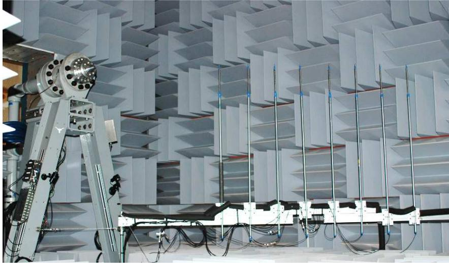
Figure 2.1: The fully anechoic chamber at UT Austin during the current set of measurements.
