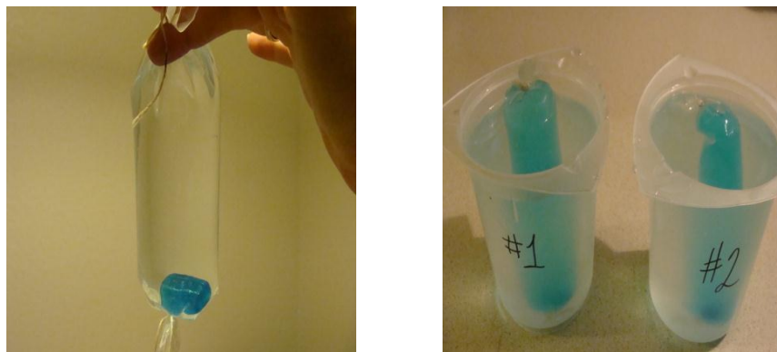
Figure 3.5 Two-Compartment Model Prototype (Dialysis tubing made into a bag to model the stomach which is compartment one. The dialysis tubing bag with candy and water in it is then submerged in water in a beaker where the beaker of water represent compartment two)
