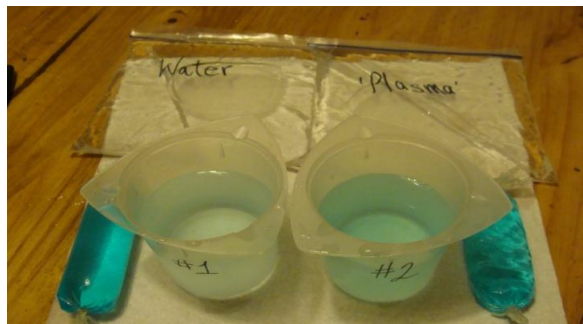
Figure 3.6 Two-compartment Model to test the encapsulation.(This is the first model to work and demonstrate proof of concept)
