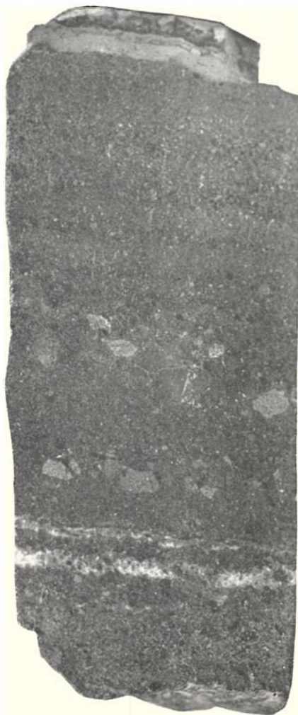
Photograph of a piece of altered igneous rock taken from Well 140. The core was secured at a depth of 1190 feet below the surface. Six-fifth natural size. Photograph by Christianson Studio.
