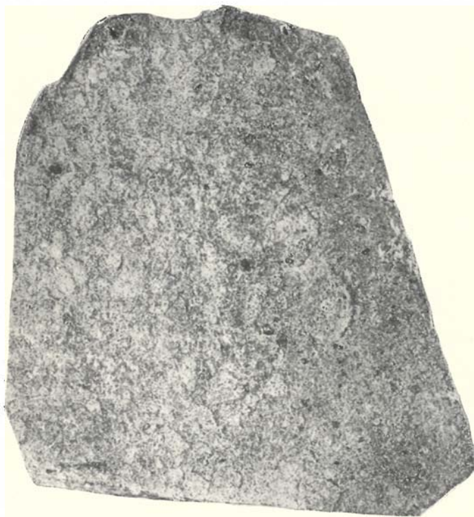
Photograph of a piece of chlorite rock said to have come from Well 164, Thrall Oil Field, at somewhere from 729 to 917 feet below the surface. The photograph shows the polished surface of the rock. Natural size. Compare this photograph with that of Plate VIII.
