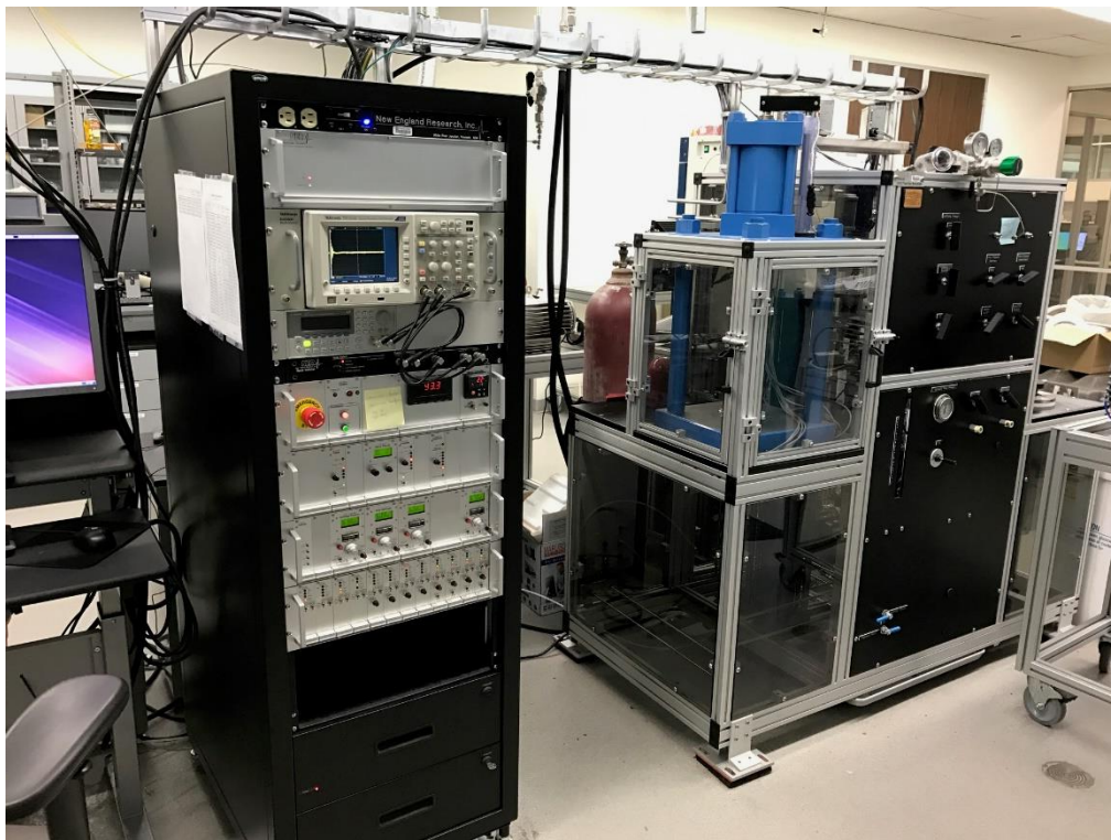
Figure C.1: Upper left: uniaxial unconfined test. Upper right: Brazilian test. Bottom: Autolab 1000 equipment used for testing.
