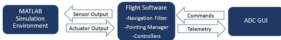
telemetry data from the ADC is displayed in the GUI, so the operator can verify that the states of the system are as expected.
