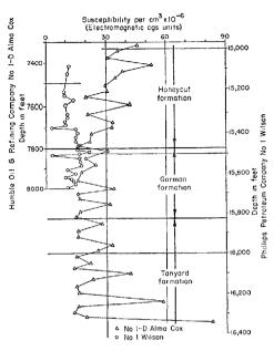
FIG. 8. Relationship of depth to magnetic susceptibility for Phillips Petroleum Company No. 1 Wilson, Val Verde County, and Humble Oil & Refining Company No. 1-D Alma Cox, Crockett County.
