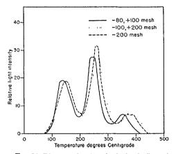
FIC. 24. Diagram showing the lack of effect of fineness of grinding on thermoluminescence properties of pre-Simpson rocks.
