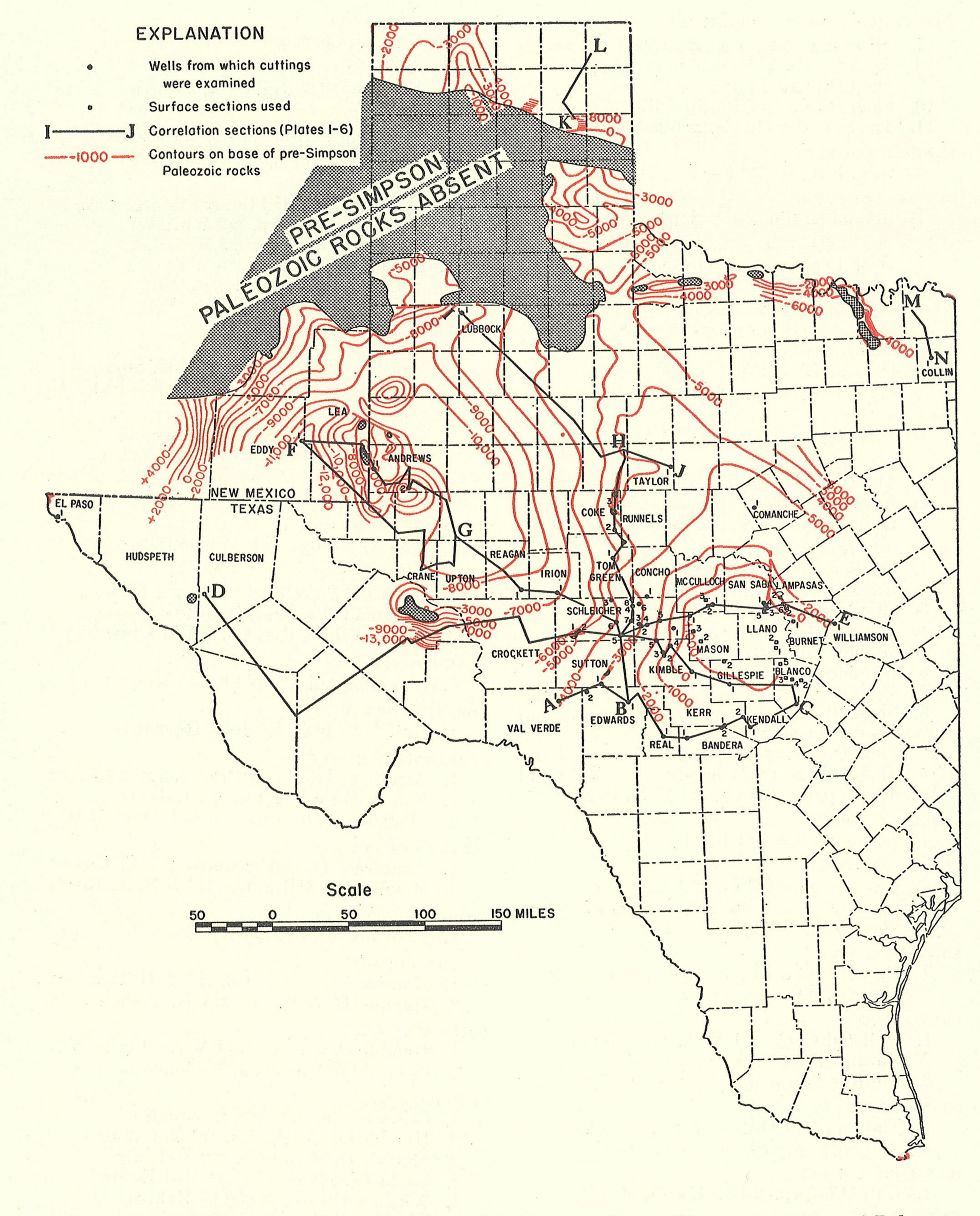
FIG. 2. Map showing present configuration of the base of the pre-Simpson sequence of Paleozoic rocks in Texas and southeast New Mexico, wells from which cuttings were examined, surface sections used either for comparison or for tests, and correlation sections.
