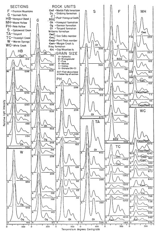
FIG. 32. Thermoluminescence glow curves of limestone from surface sections.
