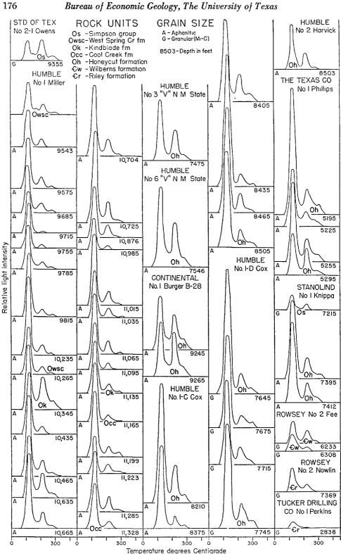
FIG. 30. Thermoluminescence glow curves of limestone, Humble Oil & Refining Company No. 1 Miller, Collin County, and various other wells as shown.
