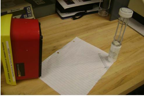
Figure 4. Ionization chamber survey meter measurement geometry configurations for both the glass vial and HDR1000 single seed holder. The 2 mm offset lines can be seen on the template for both geometry configurations.
