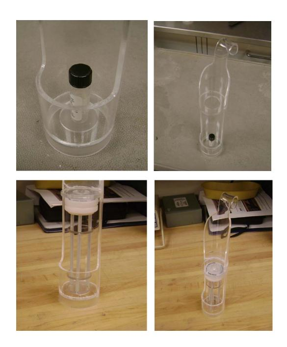
Figure 2. Geometry configurations for the glass vial and the HDR1000 single seed holder. The dippers were then slid into the activity calibrator.
