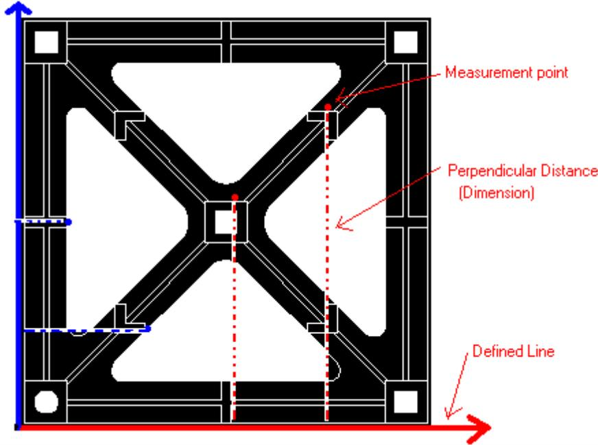
Figure:1NASUG "User Part" and the CMM measurement technique
