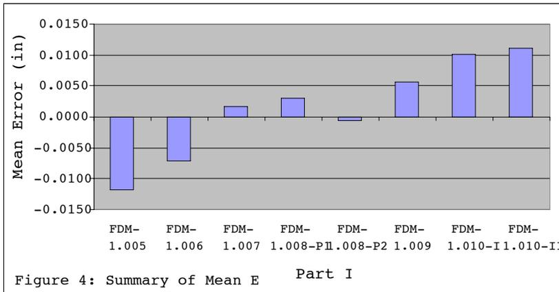
The mean error is calculated to get an indication of the error in the part and to determine whether the dimensions were within the machine specified accuracy [6]. The graph for mean error shows a similar trend to the Total Shrinkage graph and thus gives similar information. A positive mean error indicates that most of the measured dimensions were greater than the CAD dimensions, and a negative mean error indicates that most of the measured dimensions were smaller than the CAD dimensions.
