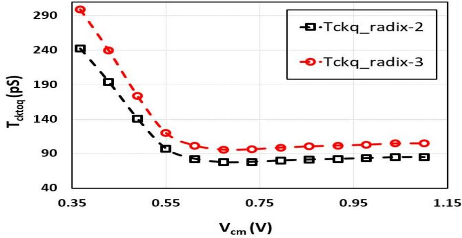
Figure 3.36: Simulated comparator clk-to-q delay at different  $V_{cm}$ .
