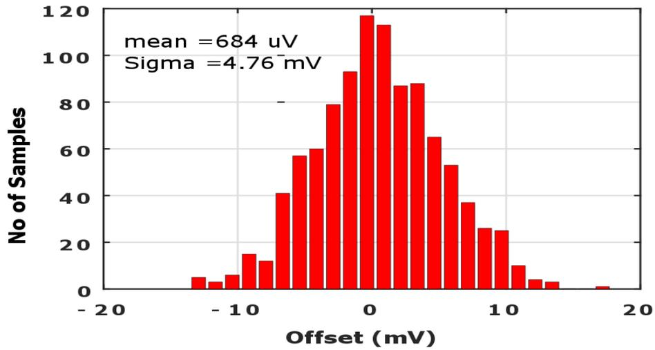
Figure 2.32: 1000-point Monte-carlo simulation for input referred offset of comparator.
