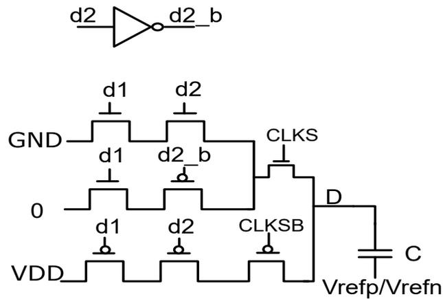
Figure 3.26: Capacitor switching with transmission gate.
