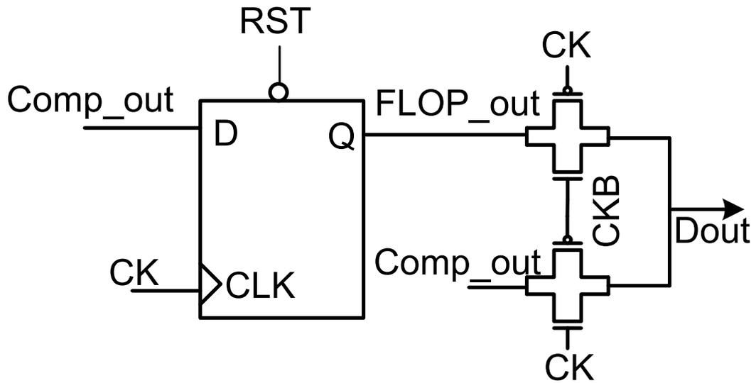
Figure 2.26: MUX circuit for radix-3 data out.
