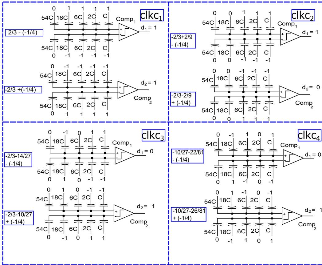
Figure 2.6: Operation example of 4-ternary-bit radix-3 SAR ADC.
