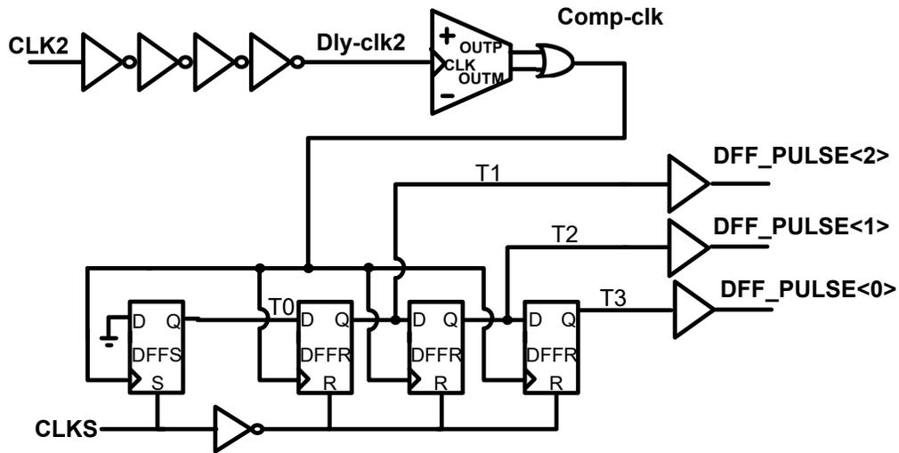
Figure 3.16: Conventional clock generation circuit for the radix-3 data flops.
