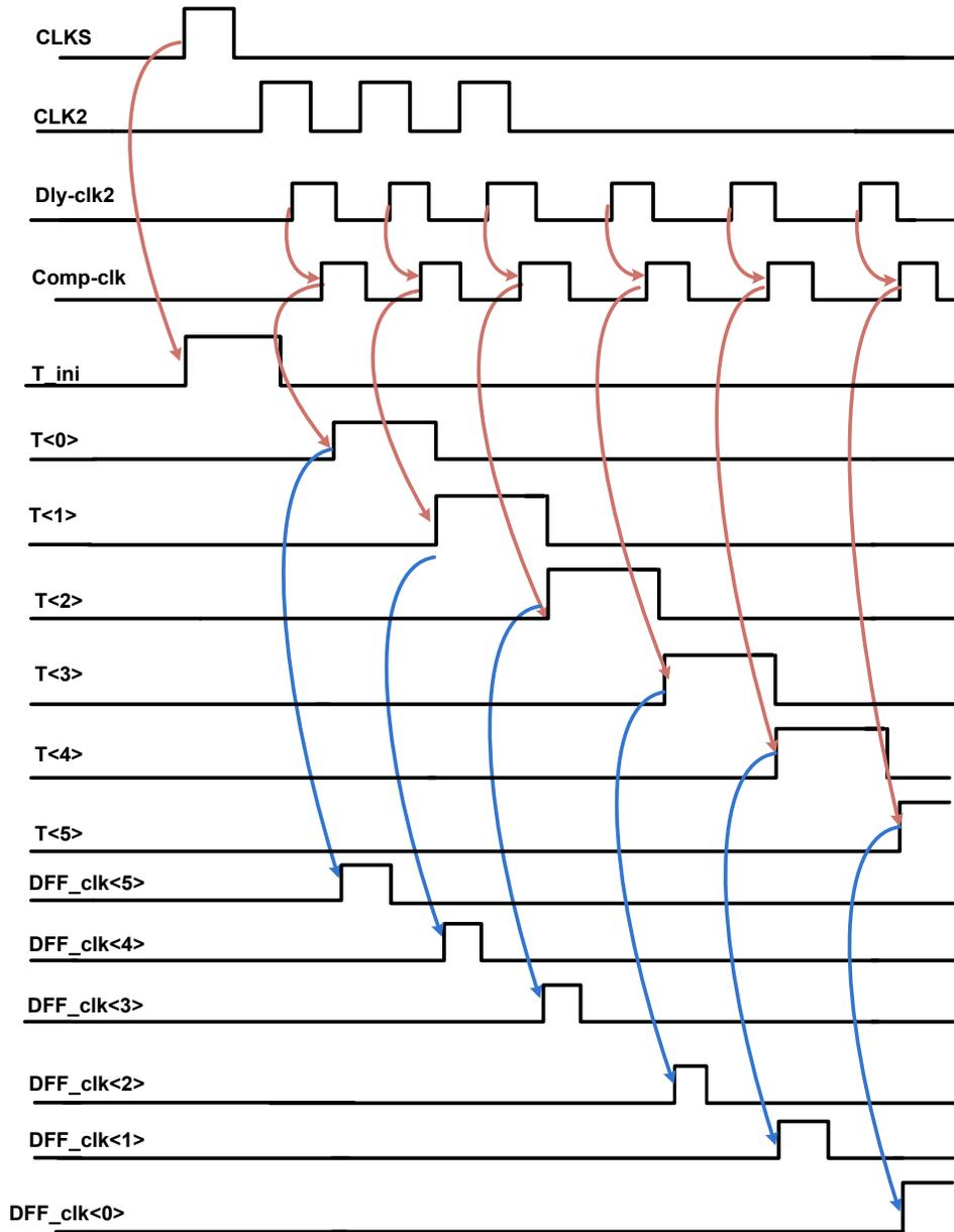
Figure 2.25: Clock generation timing diagram for 6-bit shift register.
