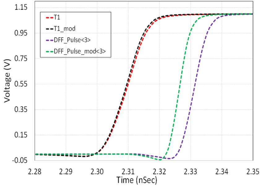
Figure 3.20: Comparison of timing between proposed and conventional scheme.
