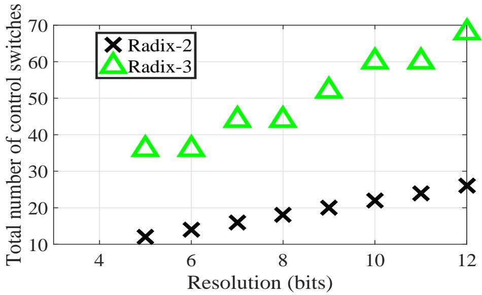
Figure 2.14: Comparison of total number of control switches.
