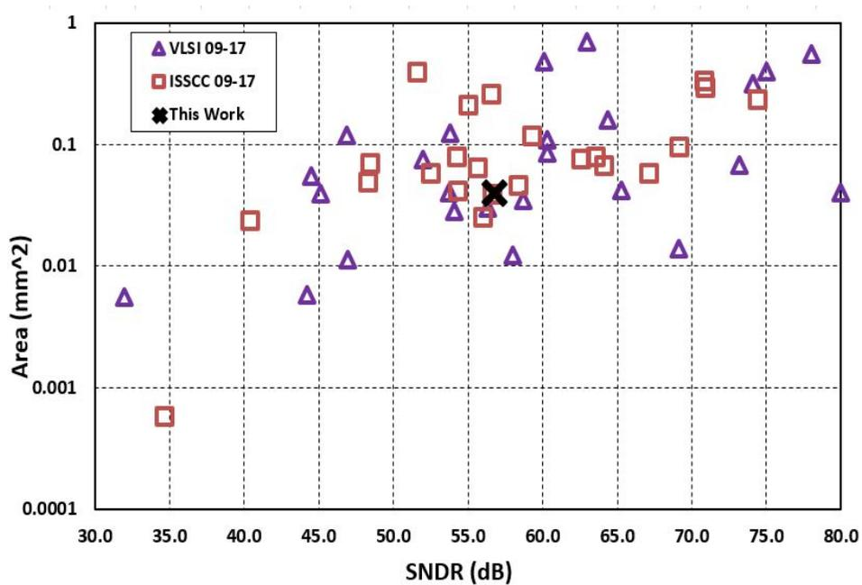
Figure 4.12: Comparison of area with ISSCC '09-'17 and VLSI '09-'17 in 40 nm CMOS process
