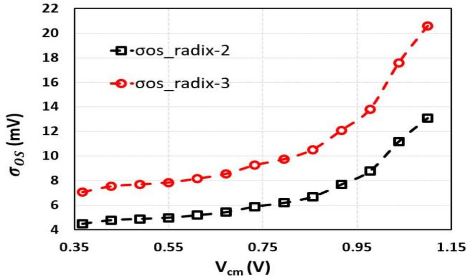
Figure 3.32: Simulated comparator offset  $\sigma$  at different  $V_{cm}$ .
