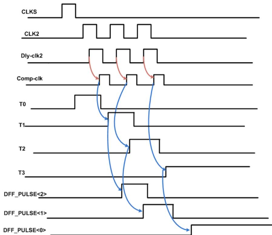
Figure 3.17: Conventional clock generation timing for the radix-3 data flops.
