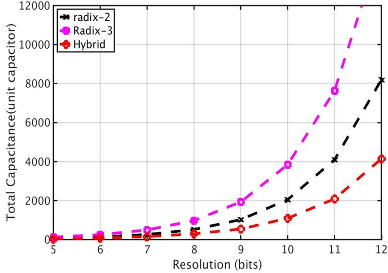
Figure 3.9: Comparison of total number of capacitors.
