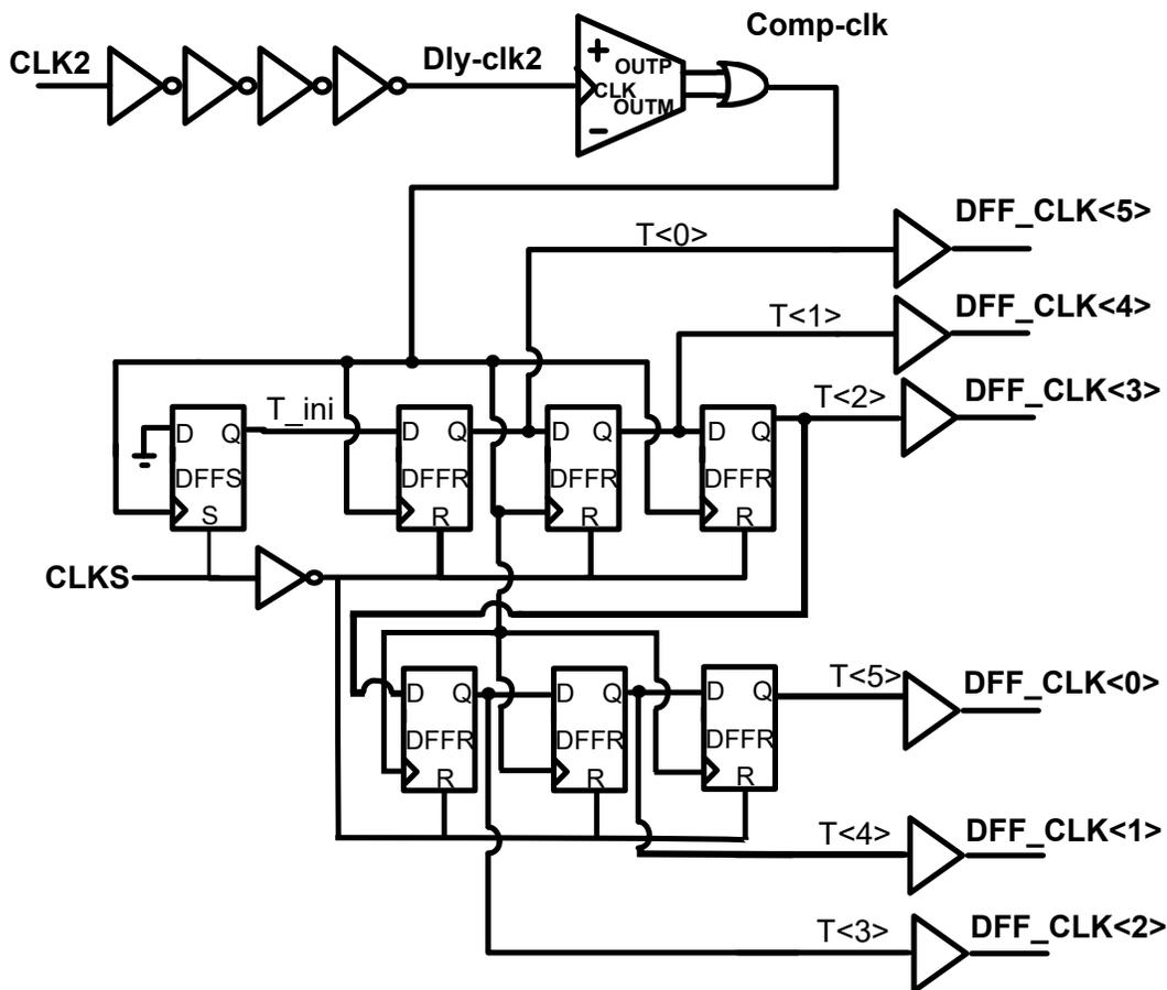
Figure 2.24: Clock generation circuit for 6-bit shift register.
