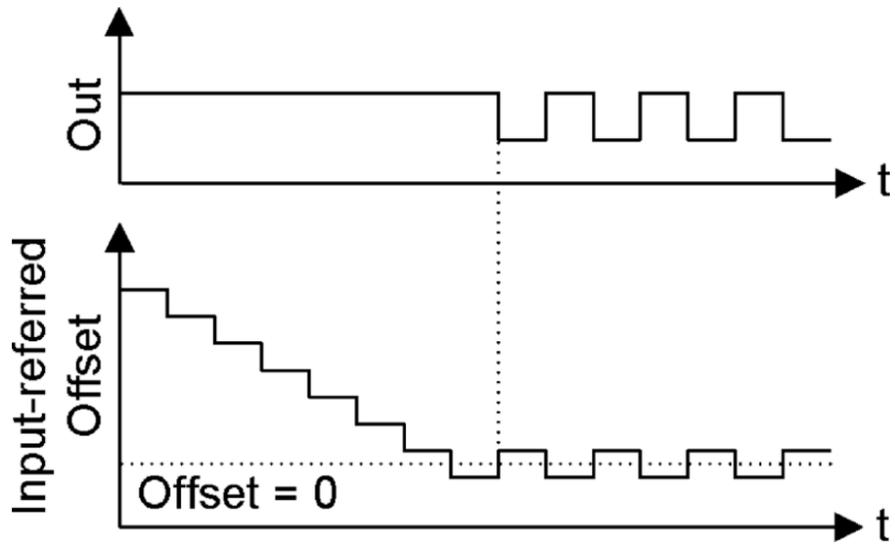
Figure 2.35: Timing waveform of change of input offset of comparator.
