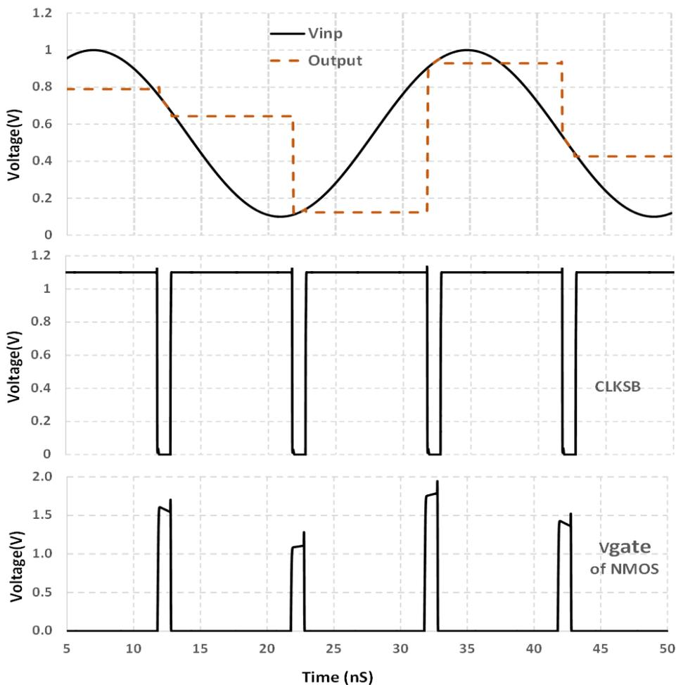
Figure 3.22: Timing diagram of bootstrapped sampling switch.
