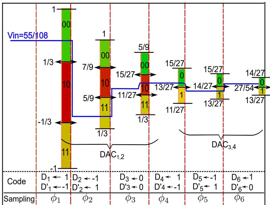
Figure 3.5: Sampling and comparison phases for (3+3) bit hybrid SAR ADC.
