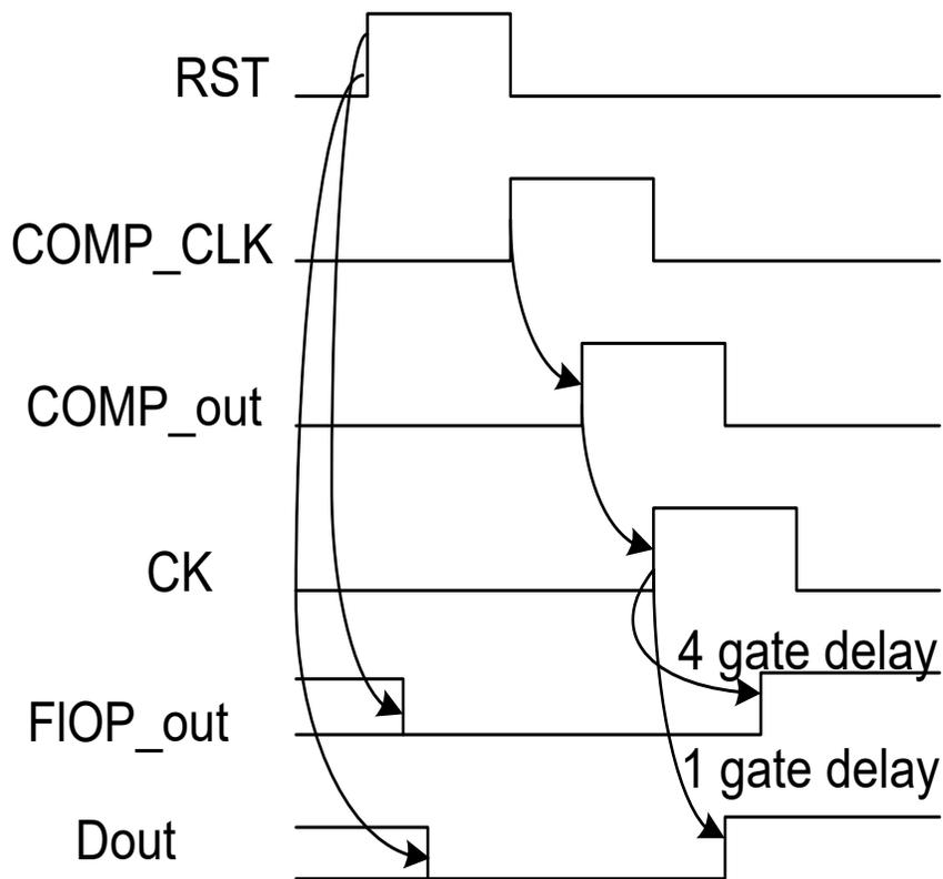
Figure 2.28: Clock to Dout delay without MUX.
