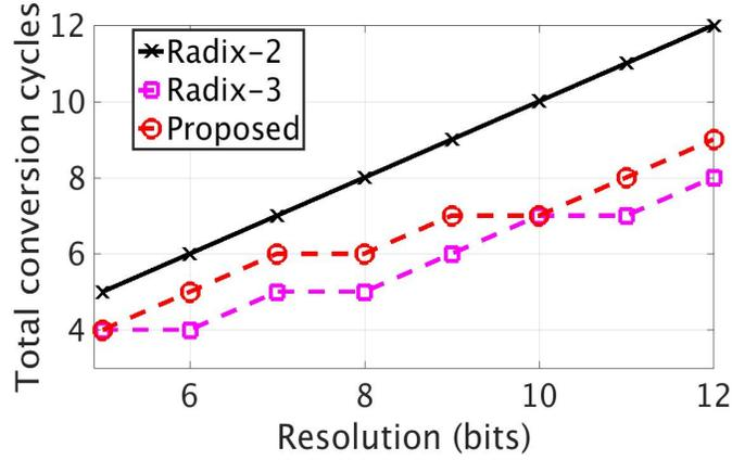
Figure 3.8: Comparison of total conversion cycles.
