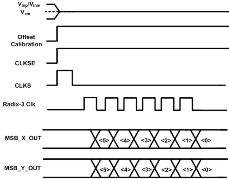
Figure 2.34: Timing waveform for calibration of comparator offset.
