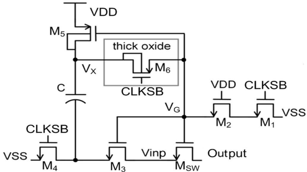
Figure 2.29: Schematic of bootstrapped sampling switch.
