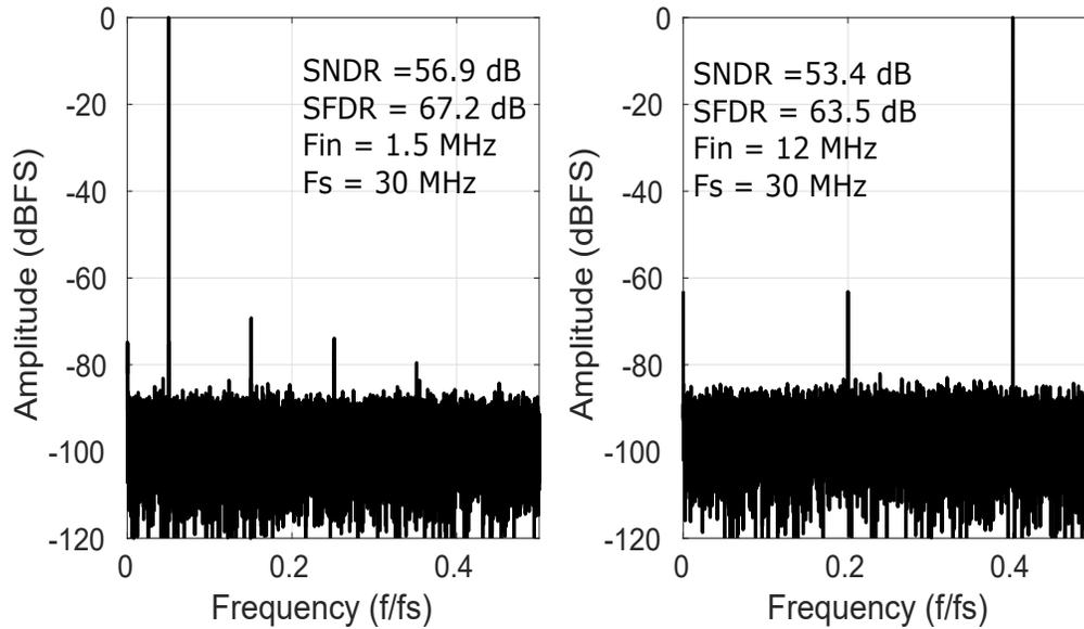
Figure 4.5: Measured 32768 point FFT spectrum with 30MS/s sampling rate and (a) 1.5 MHz input and (b) 12 MHz input.
