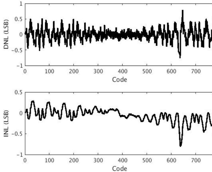
Figure 4.8: Measured DNL/INL from the designed hybrid SAR ADC.
