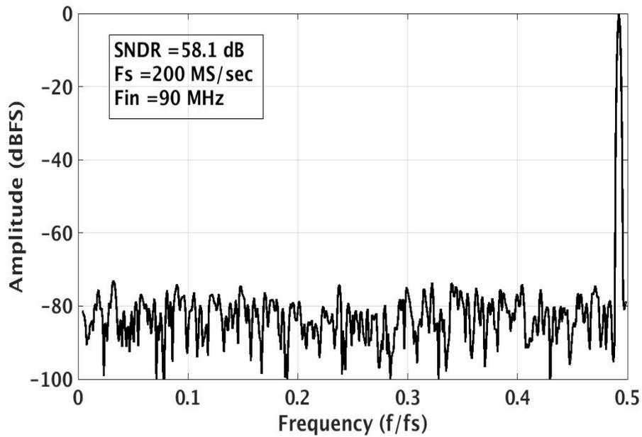
Figure 3.43: 1024 point FFT plot of the hybrid SAR ADC.
