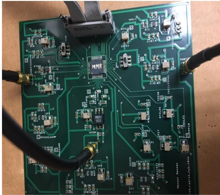
Figure 4.3: PCB setup of fabricated chip in TSMC 40nm technology.
