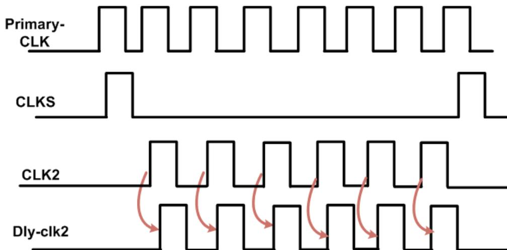
Figure 2.21: Timing diagram of the proposed radix-3 SAR ADC.
