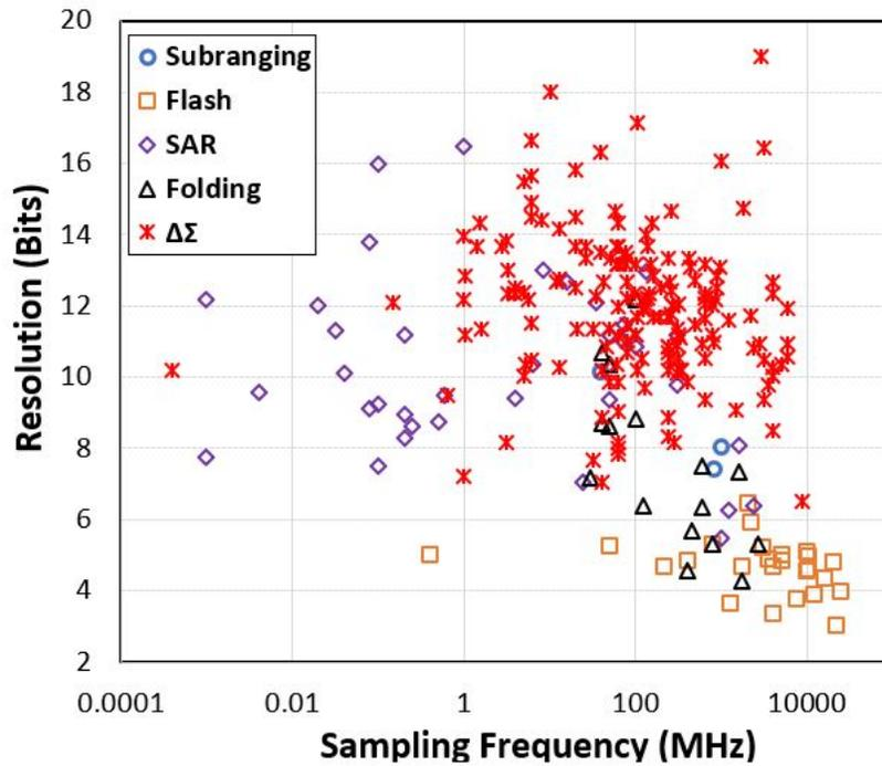
Figure 1.1: Sampling frequency versus resolution plot for recently published ADCs in ISSCC and VLSI conferences.
