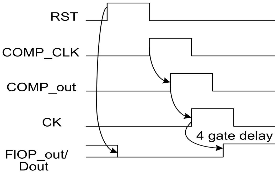
Figure 2.27: Clock to Dout delay with MUX.
