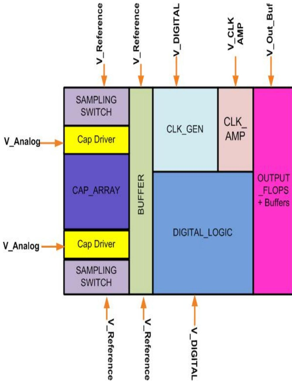
Figure 4.9: Different power sources for the hybrid SAR ADC.
