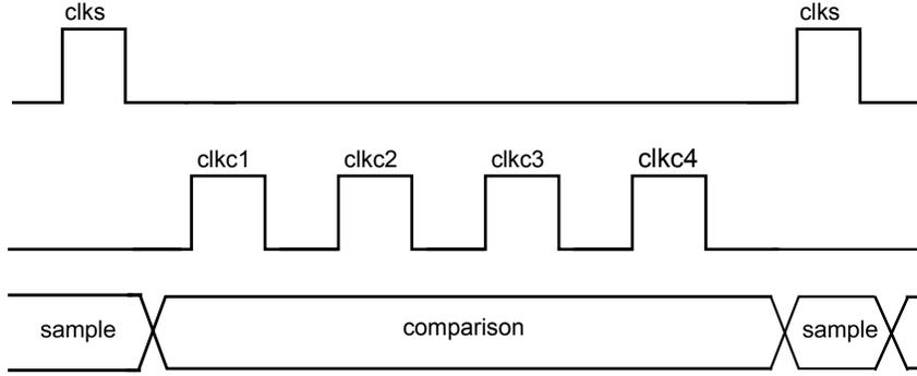
Figure 2.5: Sampling and comparison clocks for 4-ternary-bit radix-3 SAR ADC.
