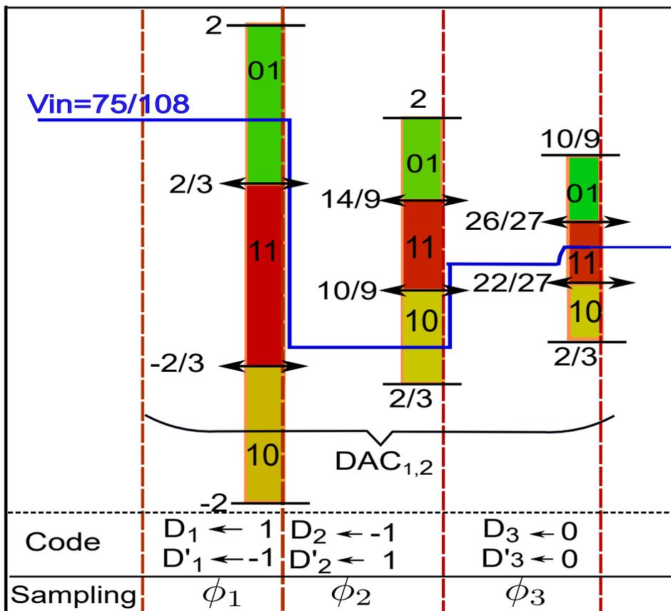
Figure 2.8: Sampling and comparison phases of 3-ternary-bit radix-3 ADC for input voltage of '75/108'.
