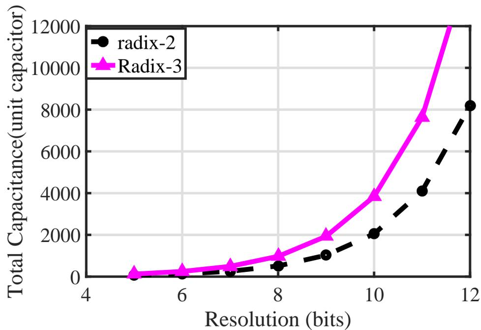
Figure 2.11: Comparison of total number of DAC capacitors.
