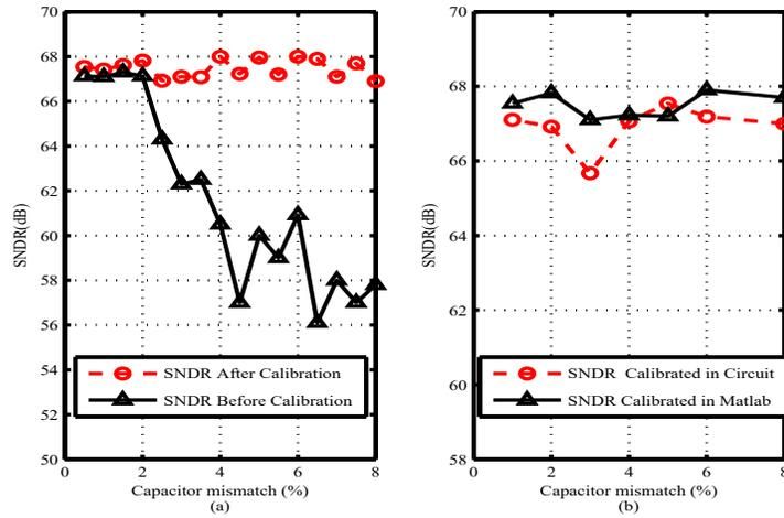
Figure 2.39: (a) SNDR of radix-3 SAR before and after calibration. (b) comparison of calibration results based on SPICE and MATLAB.
