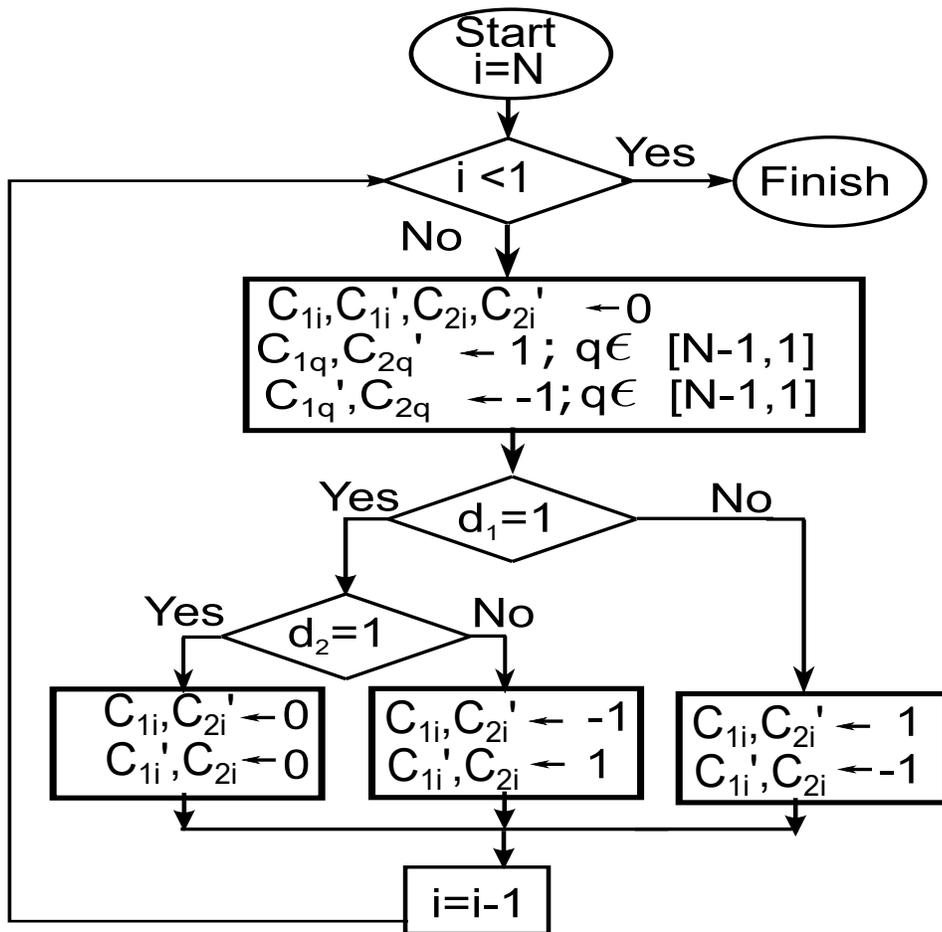
Figure 2.9: Conversion flow diagram for  $N$ -ternary-bit radix-3 SAR ADC.
