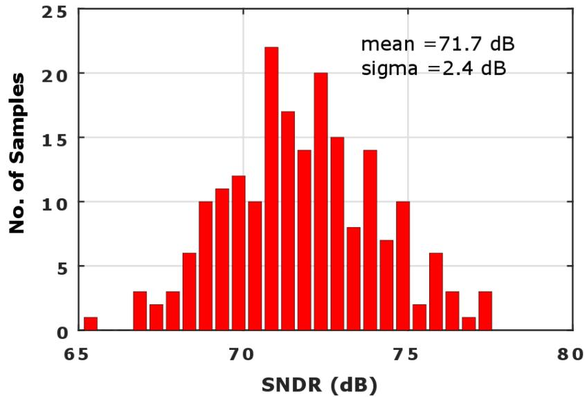
Figure 3.24: 200-point monte-carlo simulation of the bootstrapped switch frequency response.
