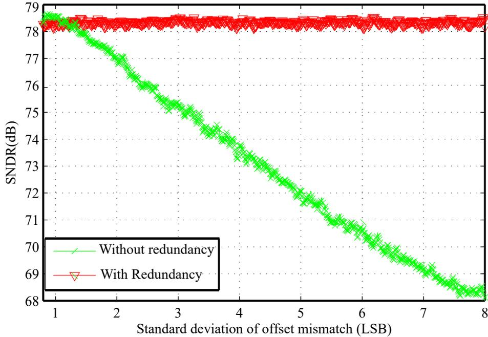
Figure 2.10: Monte-Carlo simulation to compare the effect of comparator offset.
