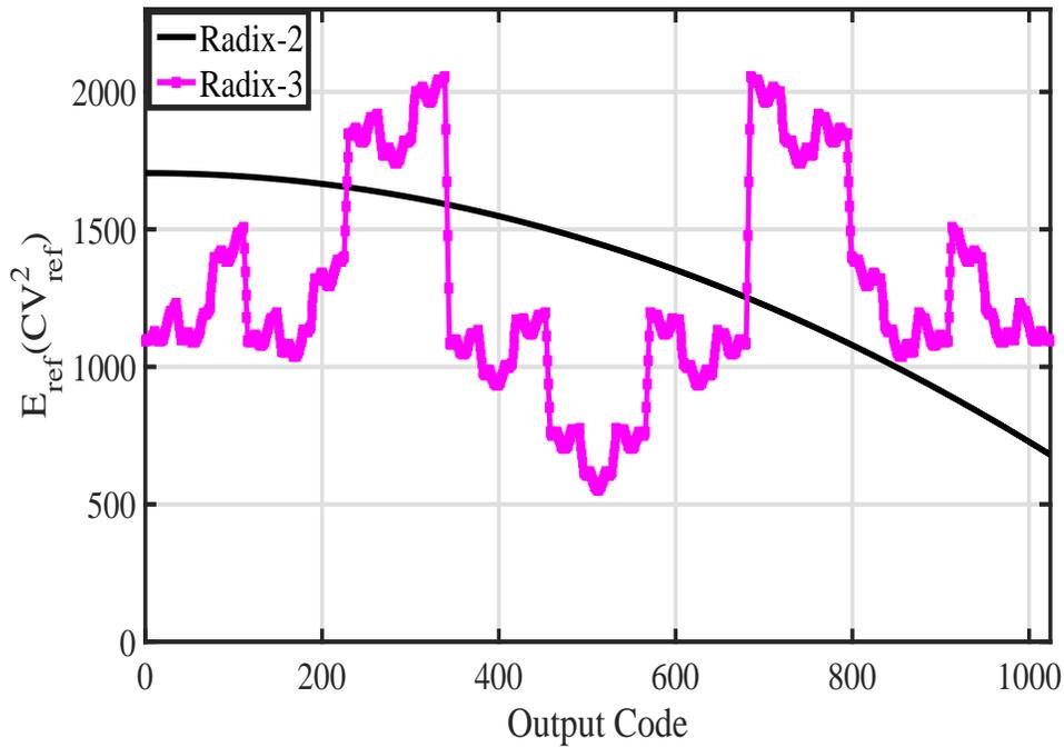
Figure 2.12: Comparison of DAC reference energy of radix-2 and radix-3 SAR ADC.
