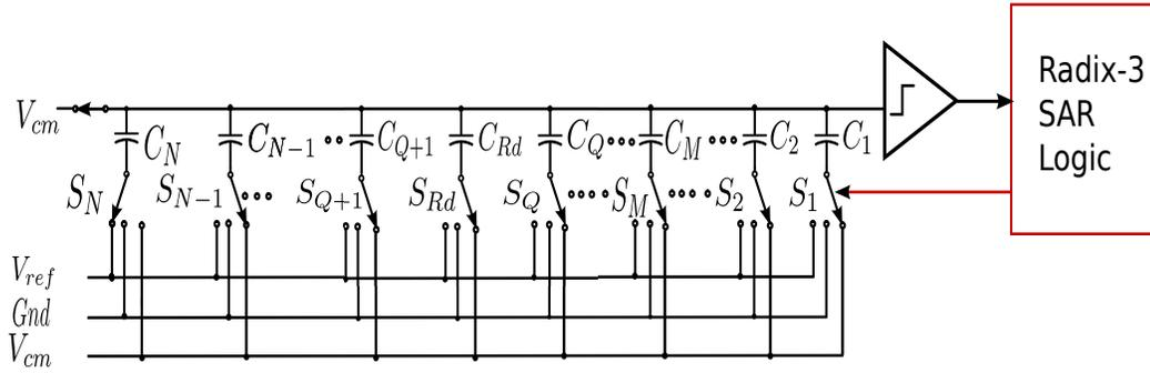
Figure 2.17: Precharging phase of calibration.
