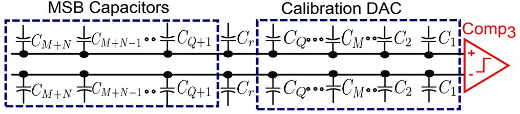
Figure 3.13: Simplified DAC of the hybrid SAR ADC.
