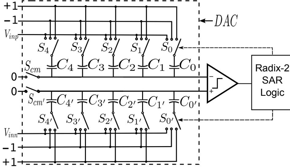
Figure 2.1: Architecture of the conventional radix-2 SAR ADC.
