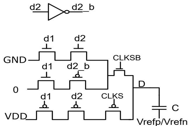
Figure 2.30: Capacitor switching circuit with transmission gate.
