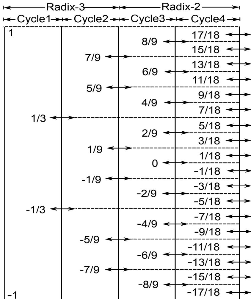
Figure 3.1: Reference voltage levels of the proposed hybrid ADC architecture.
