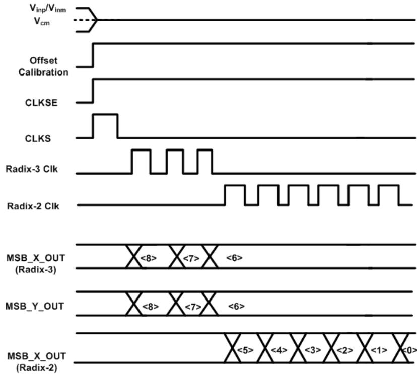
Figure 3.38: Timing diagram of comparator calibration.
