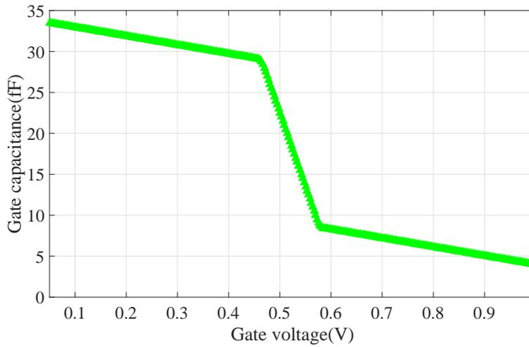
Figure 2.36: MOSFET gate capacitance variation vs control voltage.
