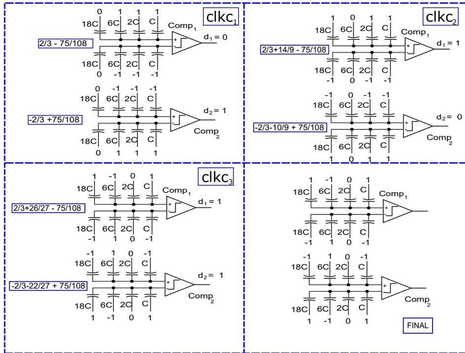
Figure 2.7: Conversion steps of 3-ternary-bit radix-3 ADC for input voltage of ‘75/108’.
