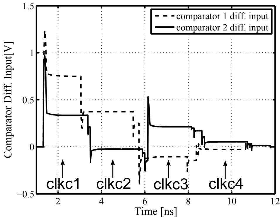
Figure 2.37: Residue voltage of 4-ternary-bit radix-3 SAR ADC.
