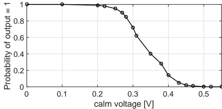
Figure 3.40: Probability of radix-2 comparator output being ‘1’ versus its *calm* with *calp* fixed at 1.1V.
