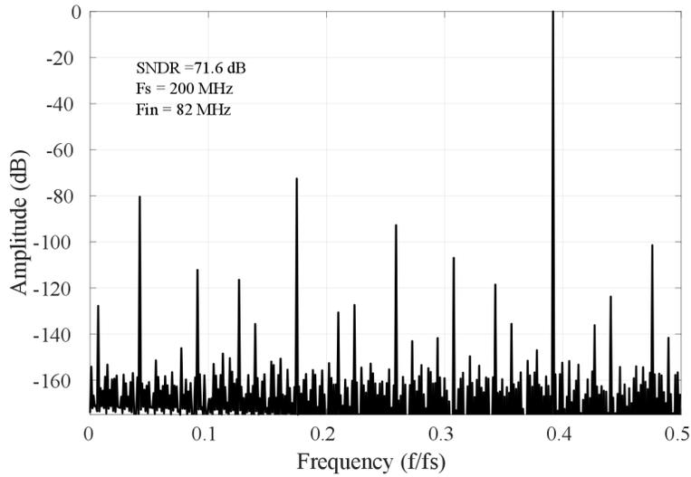
Figure 3.25: 1024-point FFT plot of the bootstrapped switch output.
