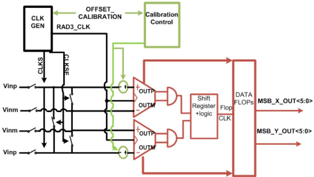
Figure 2.33: Comparator calibration scheme in proposed radix-3 SAR ADC.
