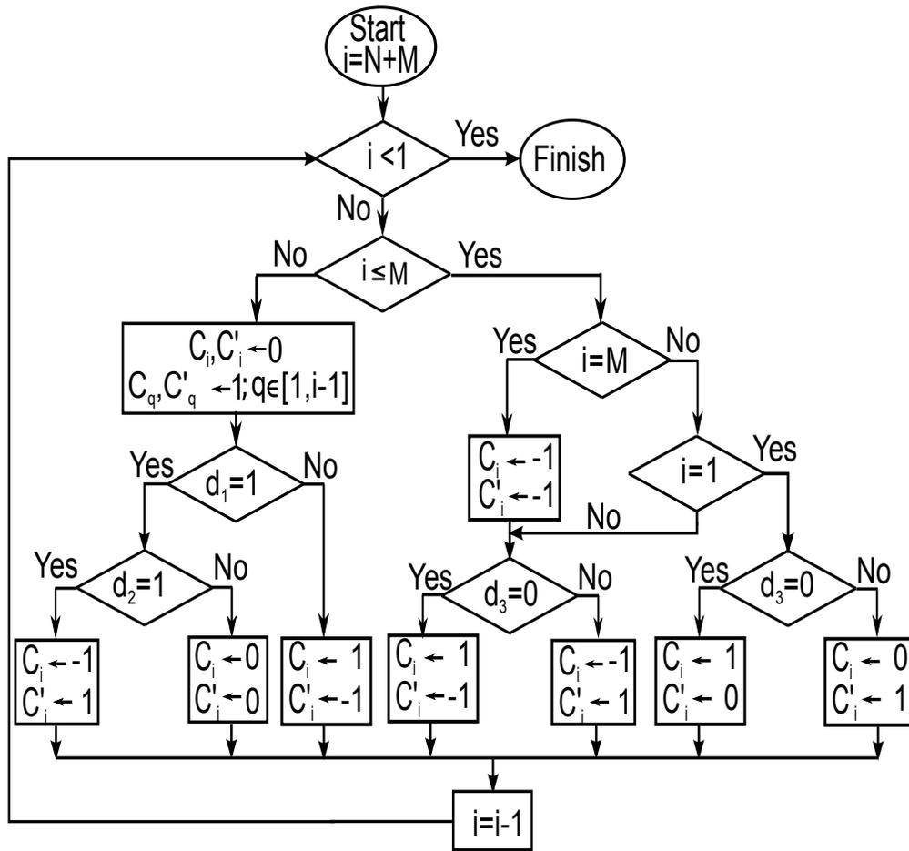
Figure 3.6: Conversion flow diagram of the proposed hybrid SAR ADC.
