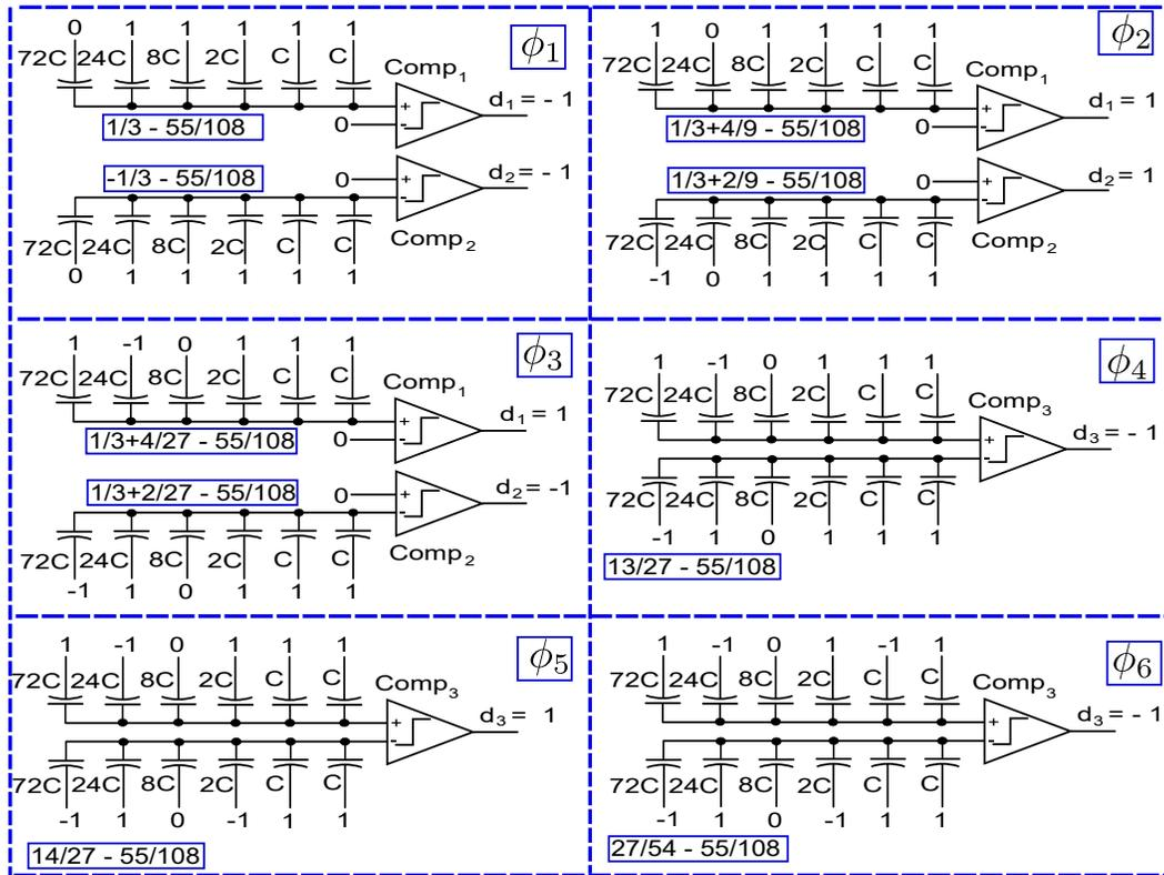
Figure 3.4: Proposed hybrid ADC's conversion steps for input voltage of '55/108'.
