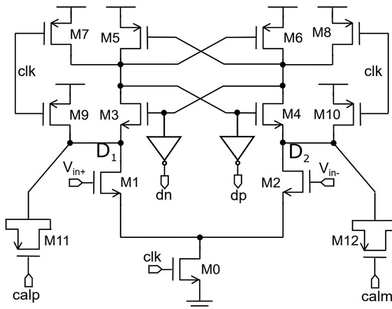
Figure 3.30: Dynamic comparator with varactor loading.
