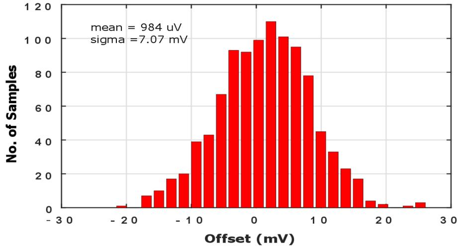
Figure 3.33: 1000-point Monte-carlo simulation for input referred offset of the radix-3 comparator.
