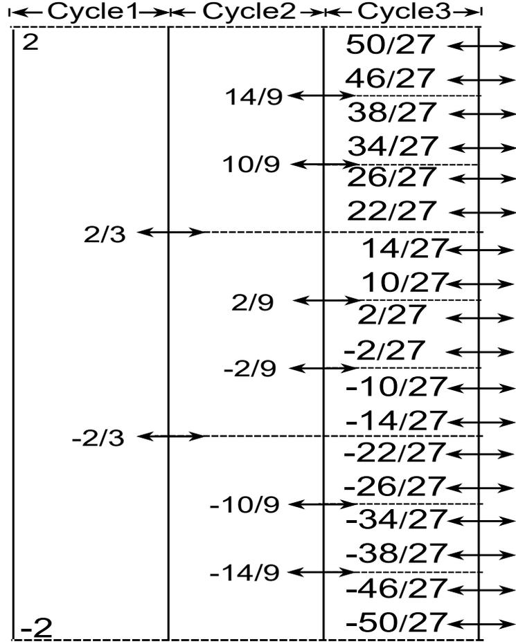
Figure 2.2: Reference voltage levels of 3-ternary-bit radix-3 SAR ADC.
