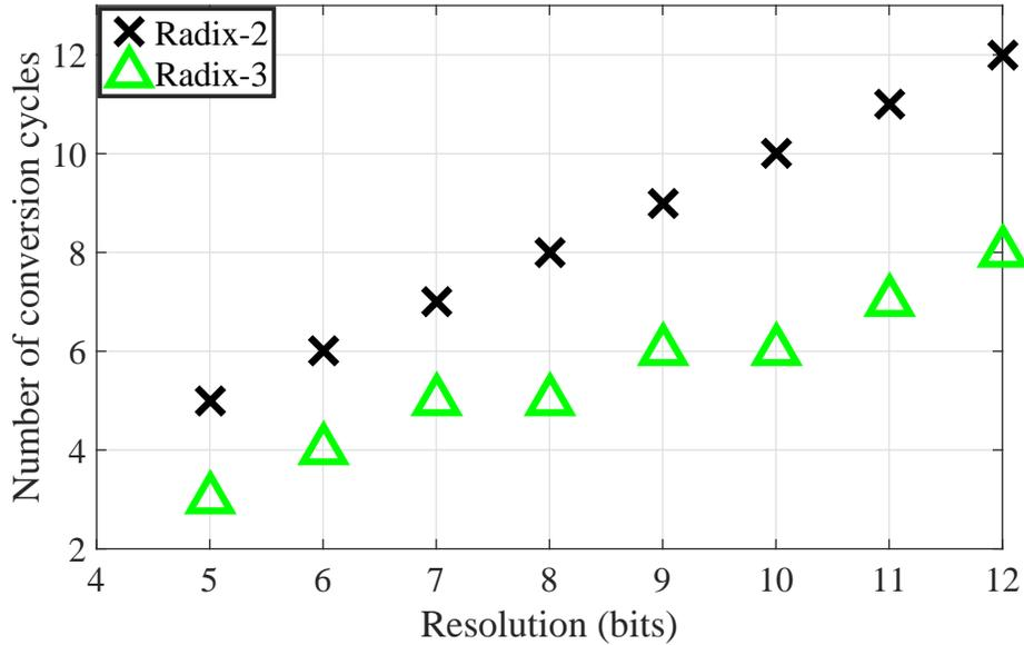
Figure 2.13: Comparison of conversion cycles of radix-2 and radix-3 SAR ADC.
