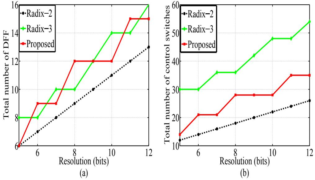
Figure 3.12: Comparison of (a) total number of DFFs (b) total number of control circuits.
