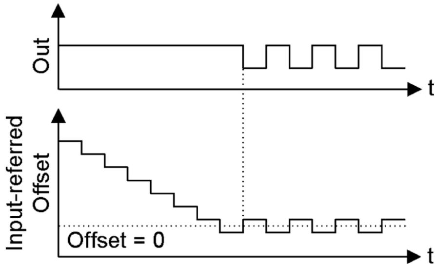
Figure 3.39: Change of input referred offset of comparators with calibration.
