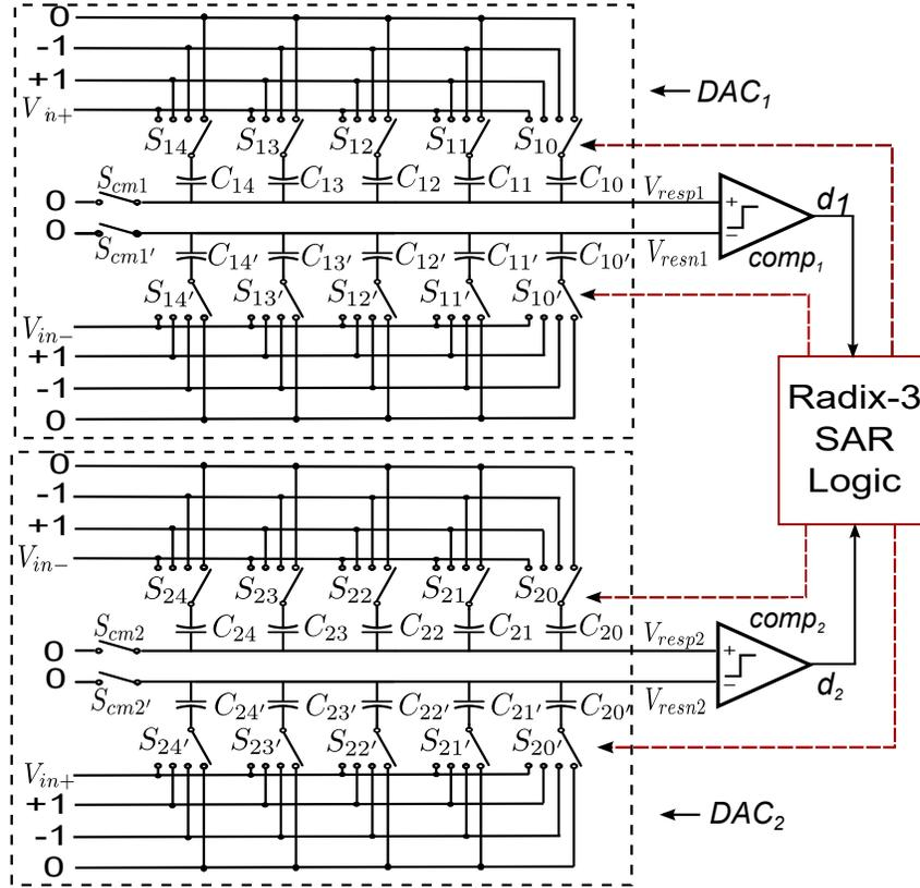
Figure 2.4: Architecture of 4-ternary-bit radix-3 SAR ADC.
