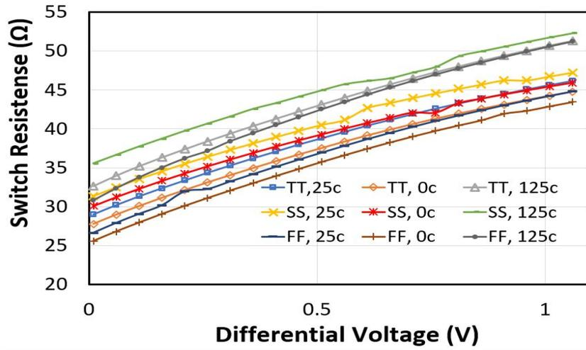
Figure 3.23: Simulated on-resistance of  $M_{sw}$ .
