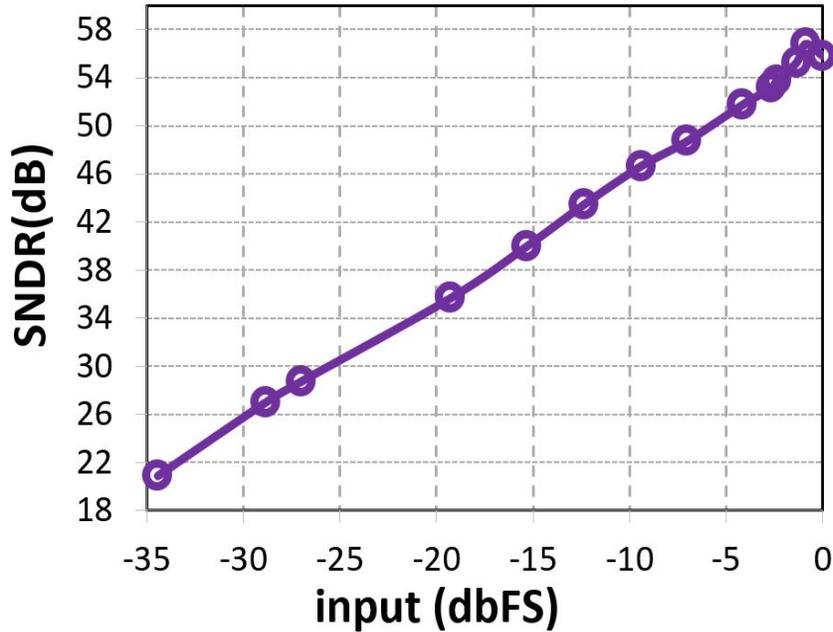
Figure 4.7: Measured linearity of the hybrid SAR ADC.
