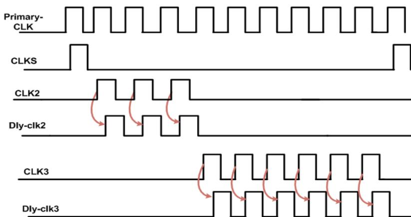
Figure 3.15: Timing diagram of the clock generation.
