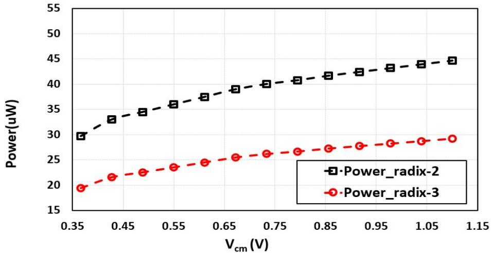
Figure 3.35: Simulated comparator power at different  $V_{cm}$ .
