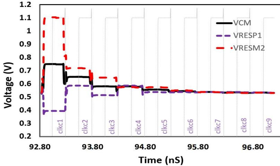
Figure 3.31: Comparator input voltage convergence and value of  $V_{cm}$  at different cycles.
