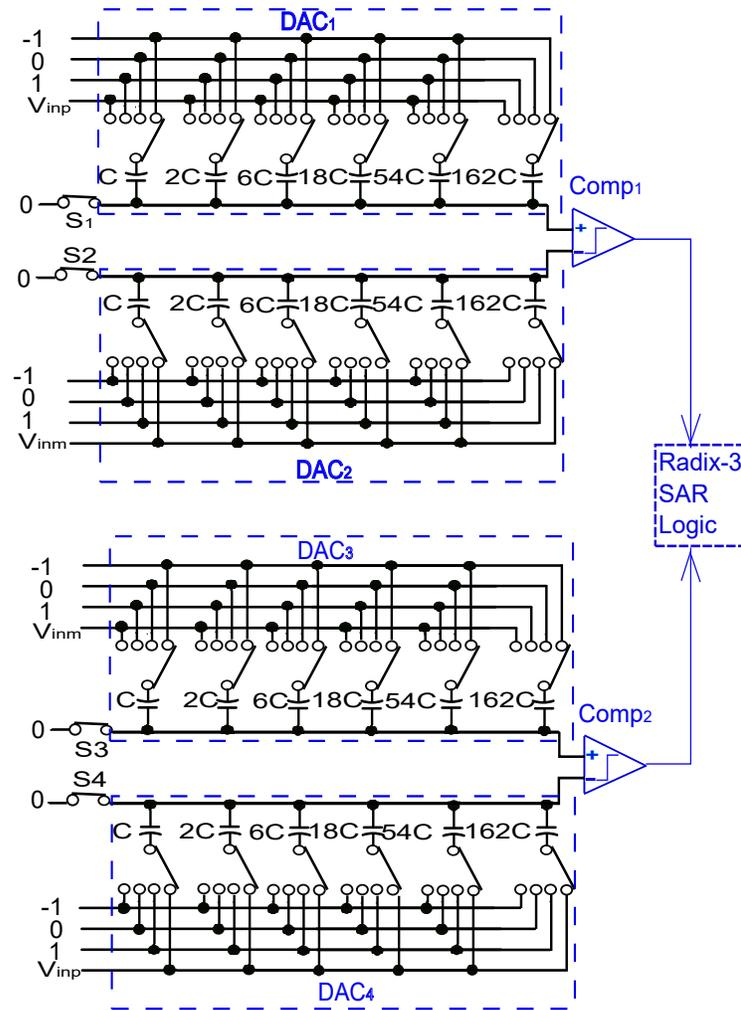
Figure 3.2: Conventional radix-3 SAR ADC.
