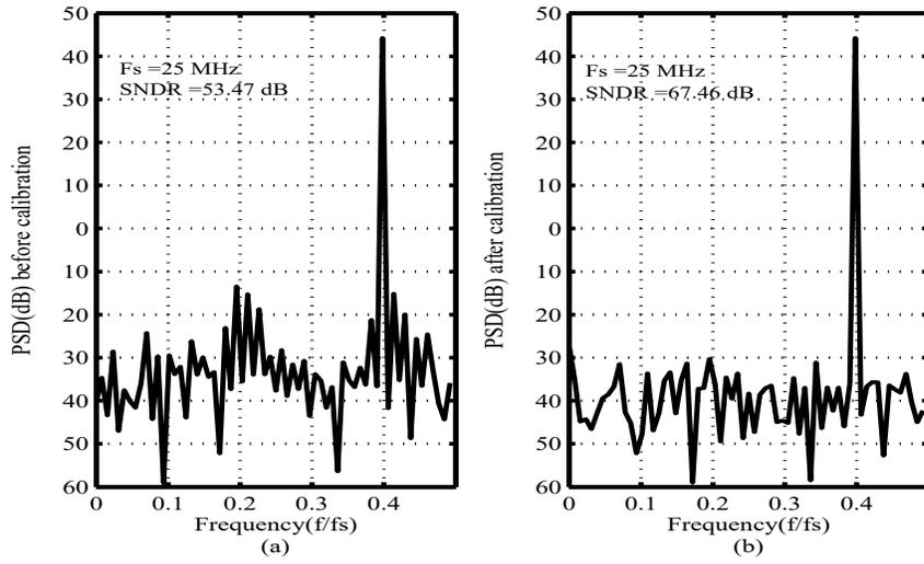
Figure 2.40: FFT of radix-3 SAR with 5% mismatch (a) before calibration (b) after calibration.
