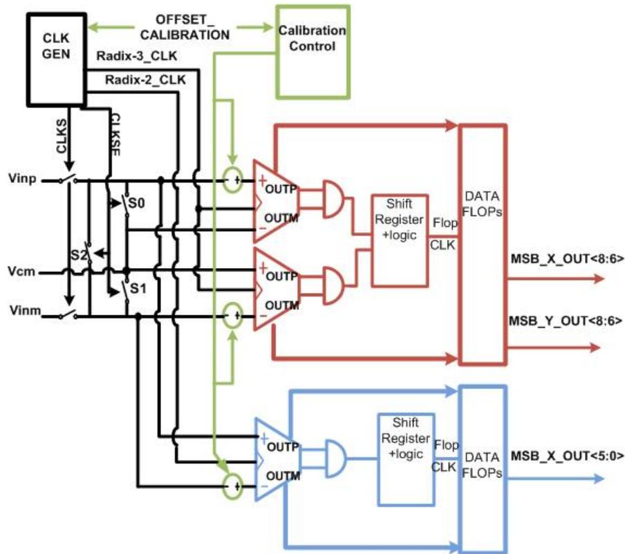
Figure 3.37: Comparator calibration scheme in proposed hybrid SAR ADC.
