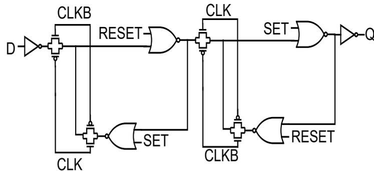
Figure 2.22: MSFF flip-flop used in radix-3 SAR ADC design.
