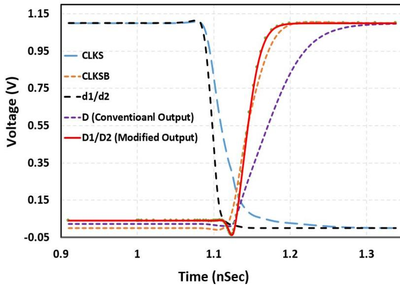
Figure 3.28: Timing diagram of the capacitor driver circuits.
