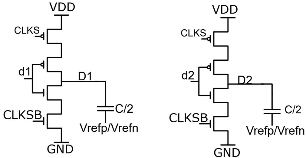
Figure 3.27: Capacitor switching with improved logic inverters.
