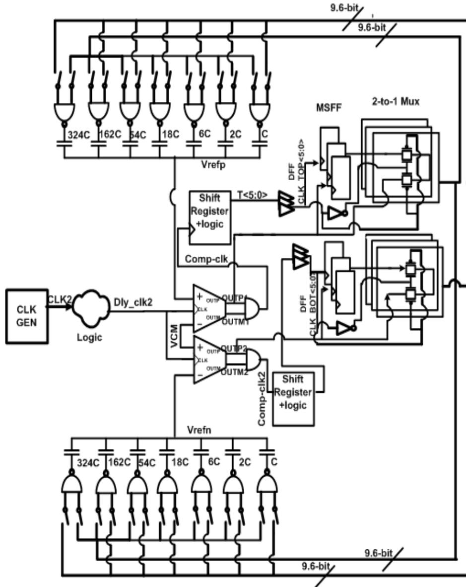
Figure 2.20: Top level circuit diagram of the proposed radix-3 SAR ADC.
