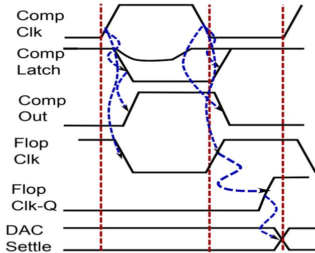
Figure 2.23: Timing waveform of MSFF.
