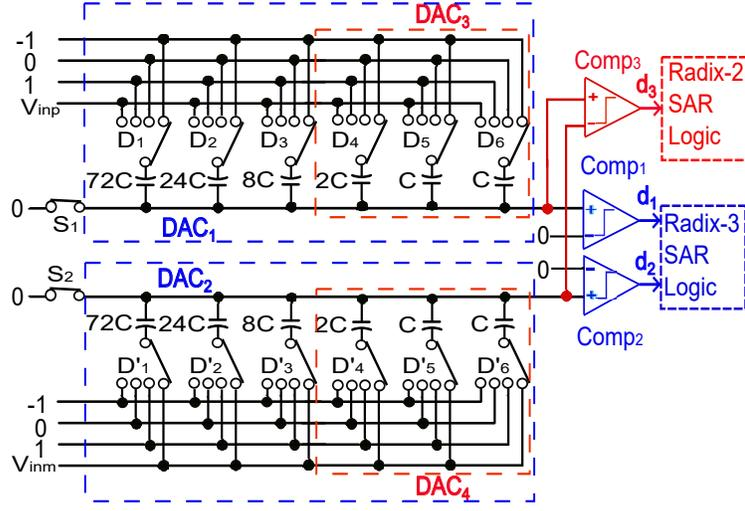
Figure 3.3: Proposed radix-3/radix-2 based hybrid SAR ADC.
