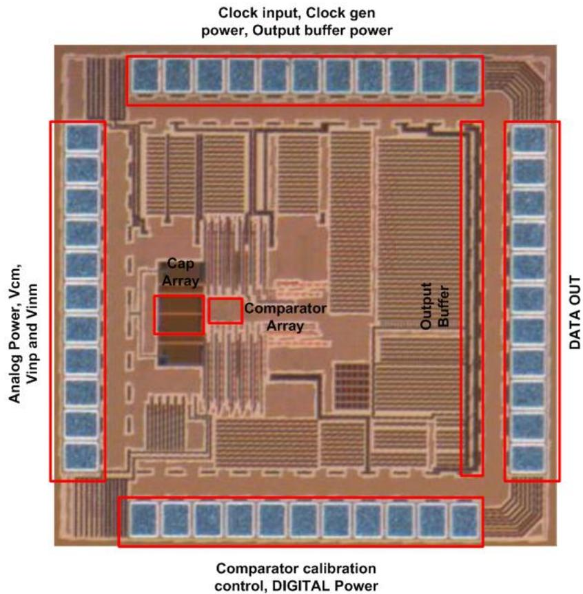
Figure 4.4: Die micrograph of the fabricated chip in TSMC 40nm technology.
