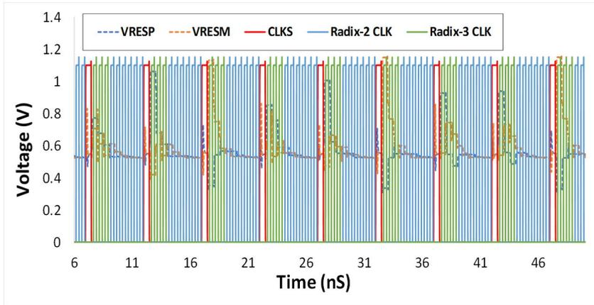
Figure 3.42: Transient simulation of the hybrid SAR ADC.
