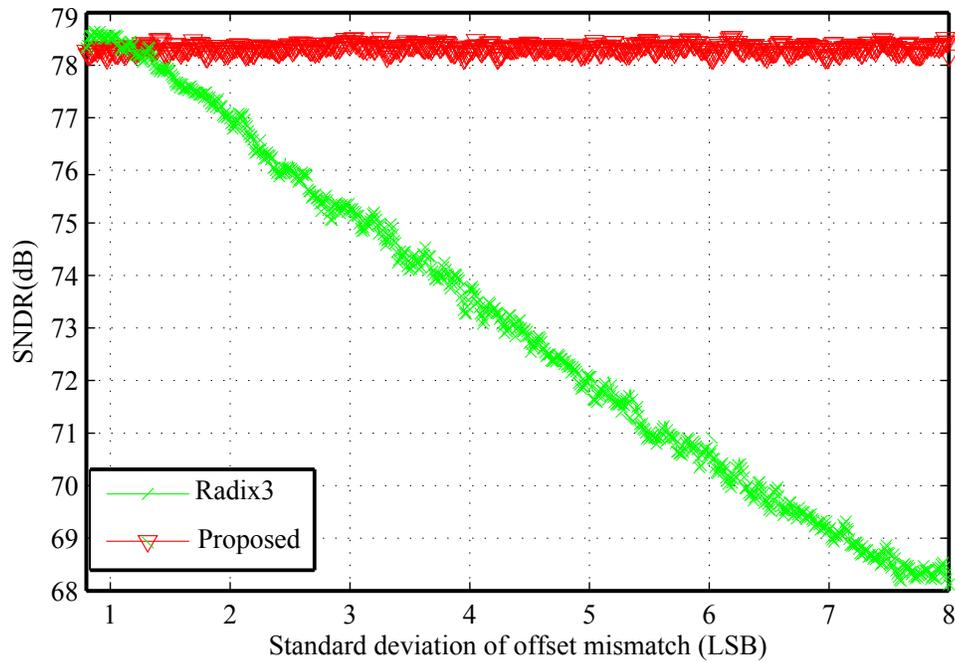
Figure 3.7: Monte-Carlo simulation to compare the effect of comparator offset.
