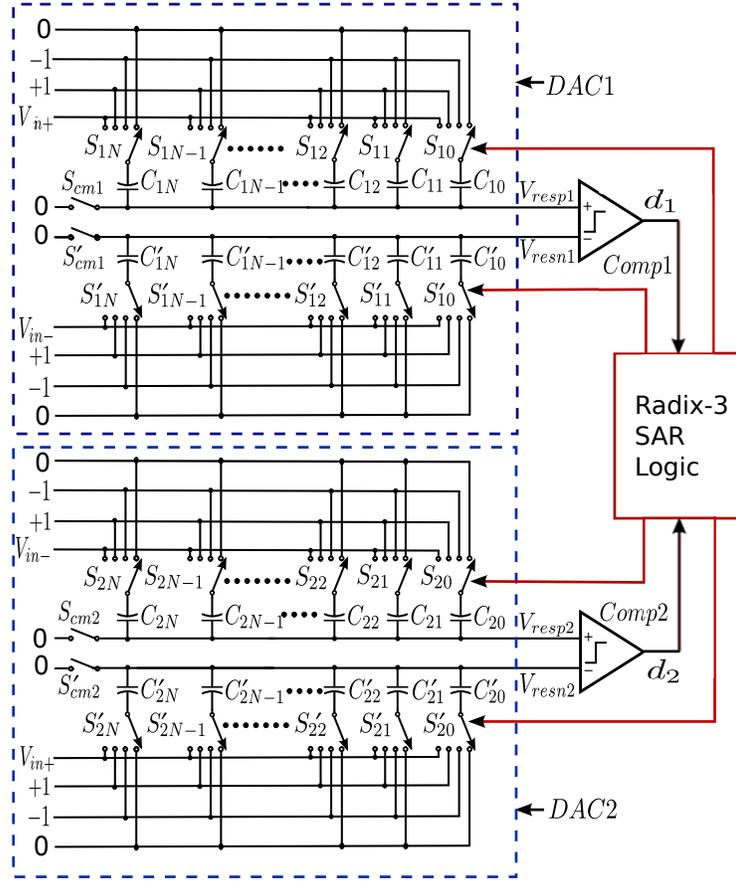
Figure 2.3: Architecture of  $N$ -ternary-bit radix-3 SAR ADC.
