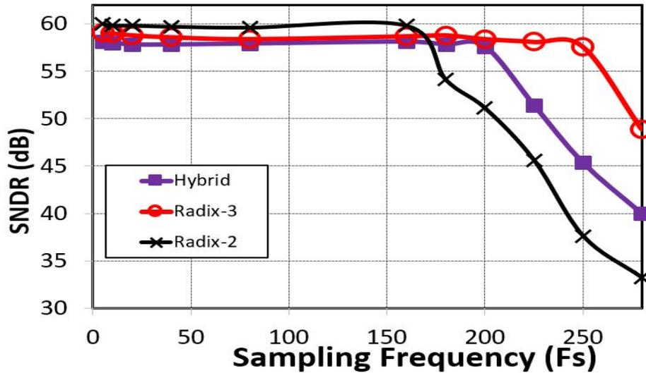
Figure 3.41: Comparison of maximum speed
