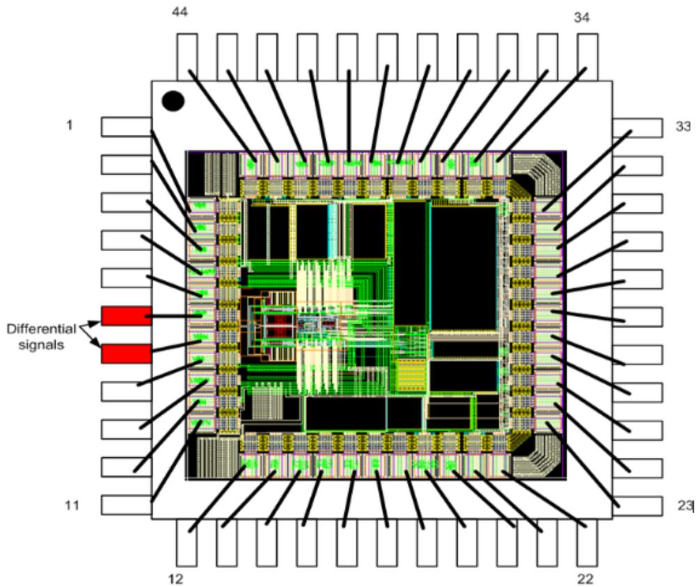
Figure 4.2: Bonding diagram of the fabricated chip.
