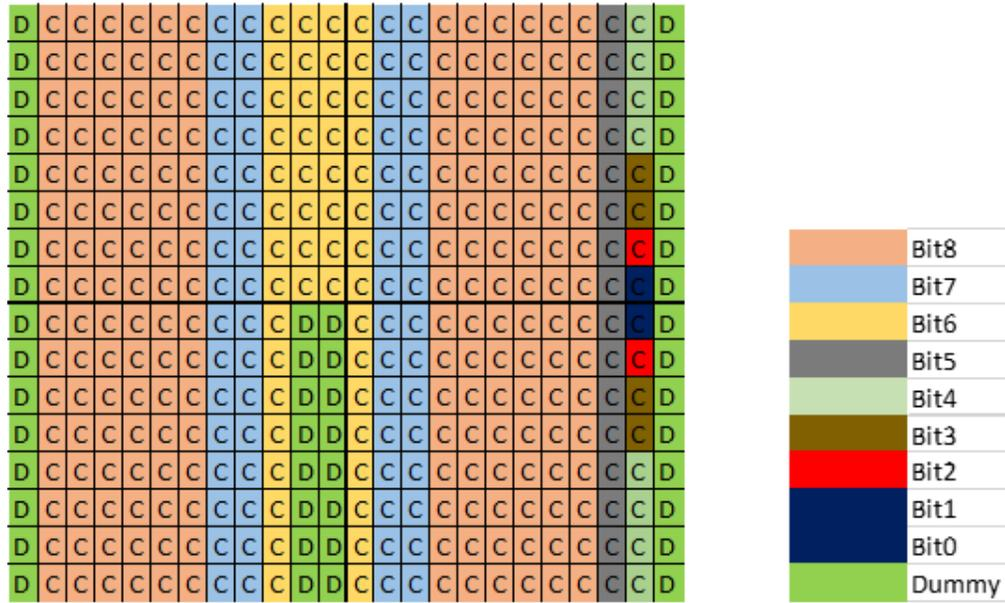
Figure 3.29: Placement of capacitor array.
