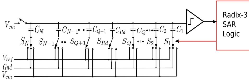
Figure 2.18: Charge distribution phase of calibration.
