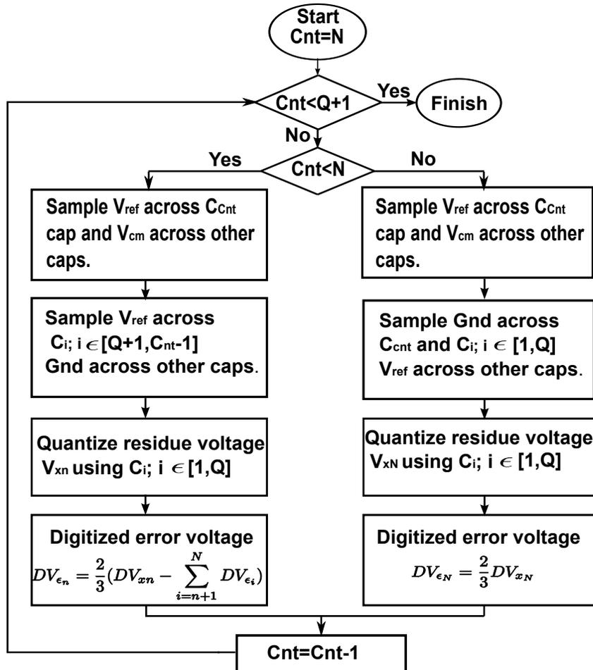
Figure 2.19: Steps for proposed calibration.
