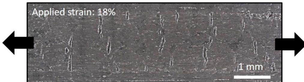
Figure A7: A global view of a Gr/PMMA ribbon on a 3M Tegaderm tape at fracture (18% of applied strain). Many macro-cracks transverse to the stretching direction is visible.
