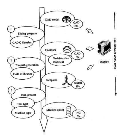
**rigure 4**: Details of process planning issues necessary in adaptive laminated machining (shown in the highlighted boxes in Figure 3).
