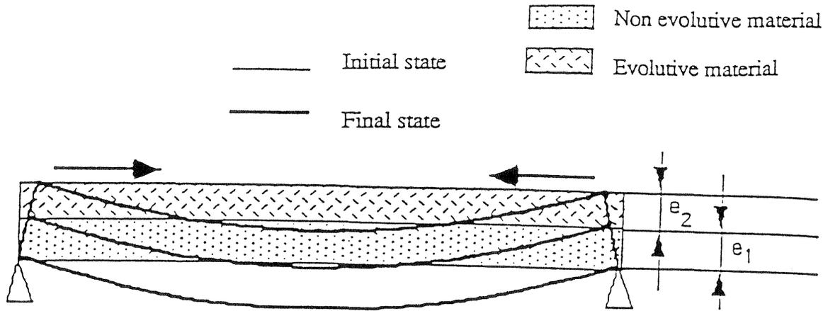
FIG. 3: Deformation induced by resin shrinkage (Simulation)
