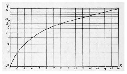
The length of the perpendicular from any point, 6 for example, up to the curve, gives the proper relative interval 1-6 on the Slide Rule. Consequently, if we have a 10-inch rule (the usual length) and imagine it to be divided into 100 equal parts, we will find from the properly constructed curve that if the starting point is numbered 1, then at the end of 301 parts we should put the figure 2; at the end of 602 parts, the figure 4; and at the end of 903
