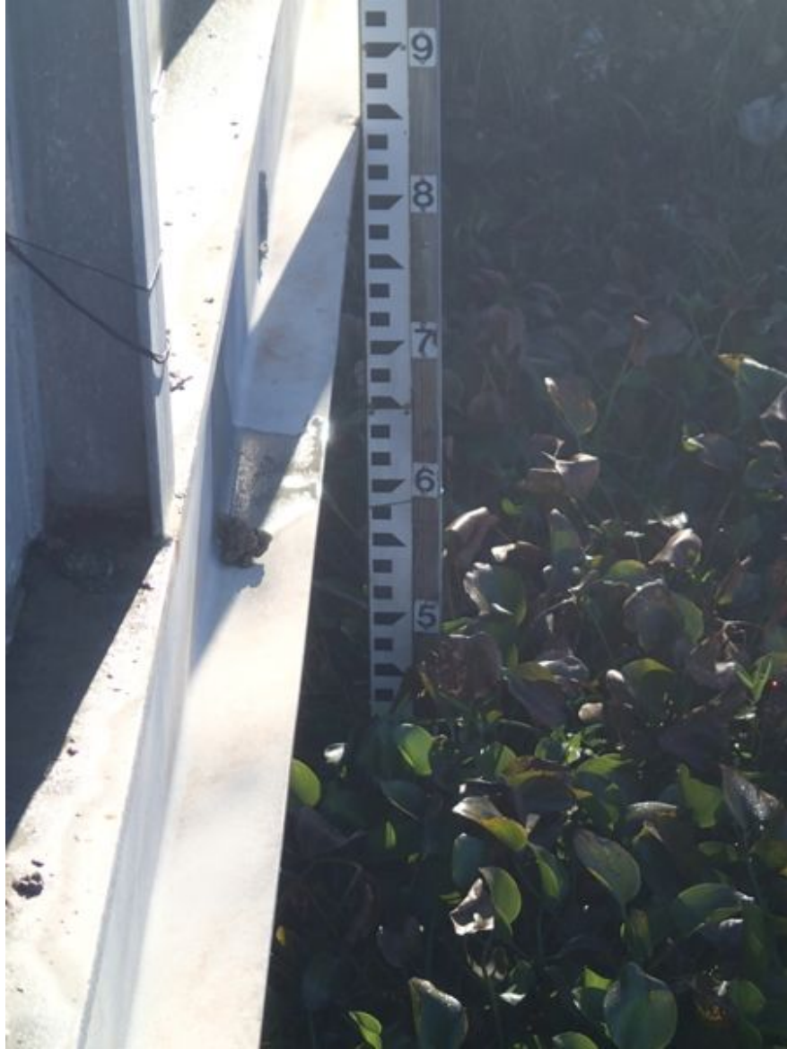
Figure 12. Water level gage on diversion canal from bridge that is accessible off TX-35 (wp04). Photograph by Ben R. Hodges, ©2013. File wp004 bSSE BridgeOverDiversionChannel i038.
