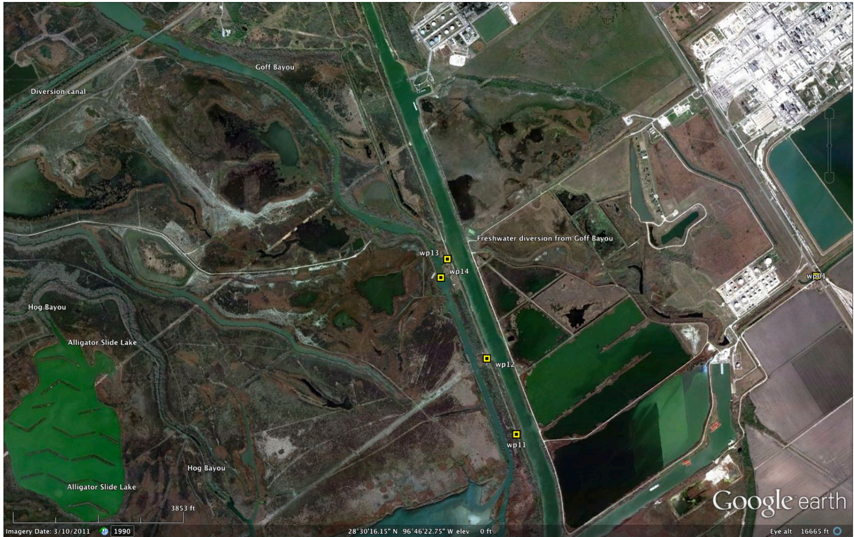
Figure 21. Goff Bayou connection with diversion canal and Mission Lake. Note the freshwater diversion from wp13 goes underneath the Victoria Barge Canal and connects to industrial supply canals to the east of the barge canal. Imagery from Google Earth dated 3/10/2011.
