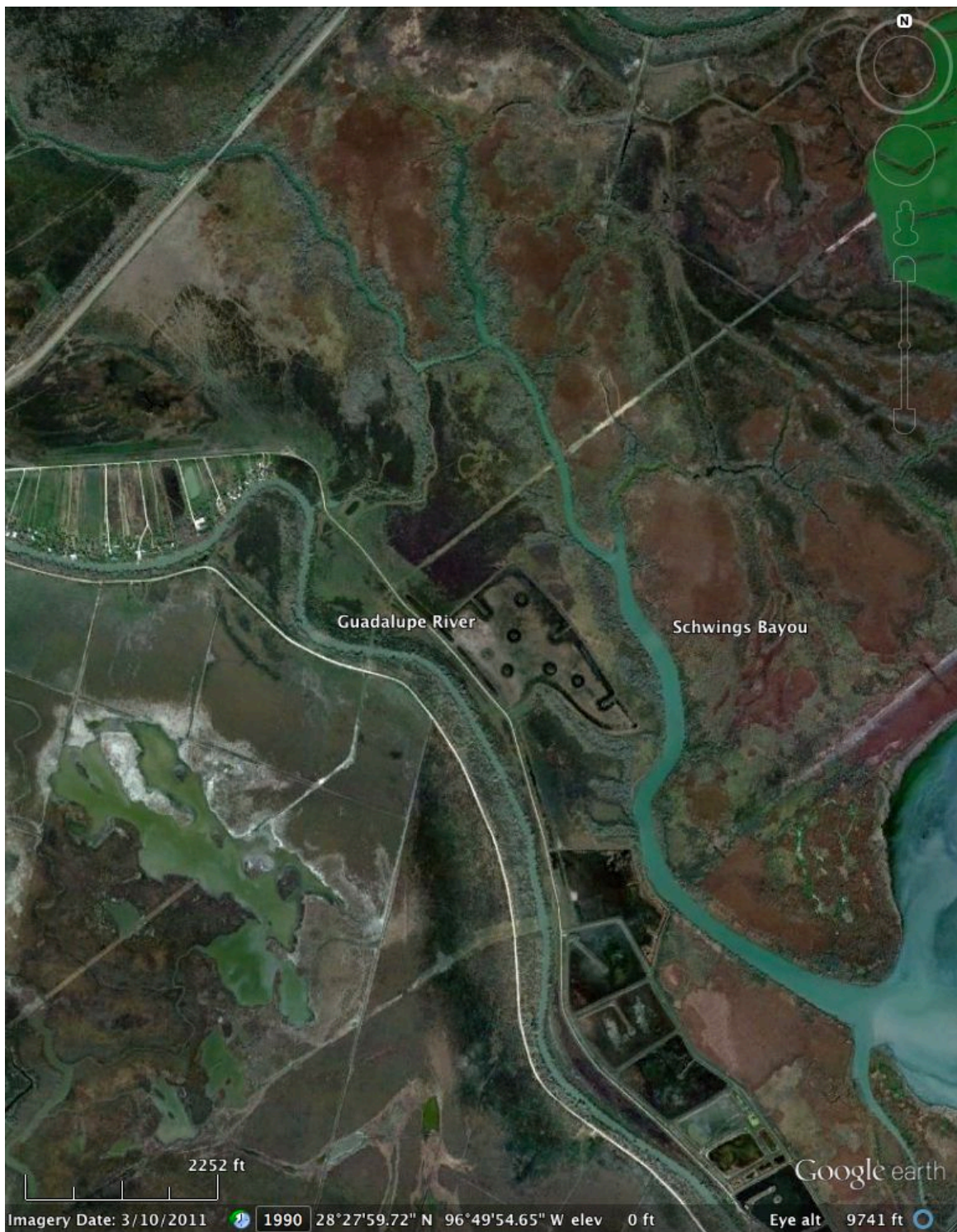
Figure 14. Schwings Bayou. Note that this bayou does not have a surface water connection to either the Guadalupe River upstream of the salt barrier or the diversion canal. There is apparently a culvert connection near the river bend. There are no significant blockages for upstream exchange of marine water. Imagery from Google Earth dated 3/10/2011.
