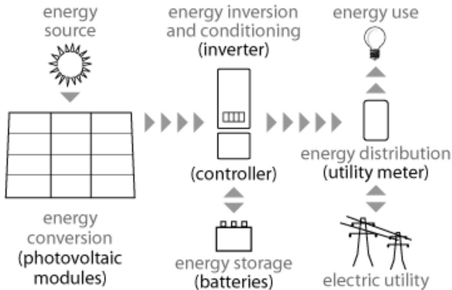
Source: Solar Direct, “Complete Photovoltaic Systems,” <http://www.solardirect.com/pv/systems/systems.htm>.
