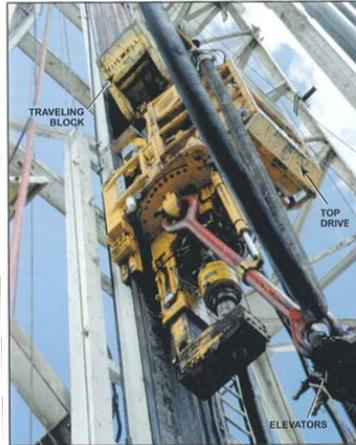
Figure 3.4: The top drive is suspended from the traveling block, and axial position is set through manipulation of the block speed. [Bommer, 2008]
