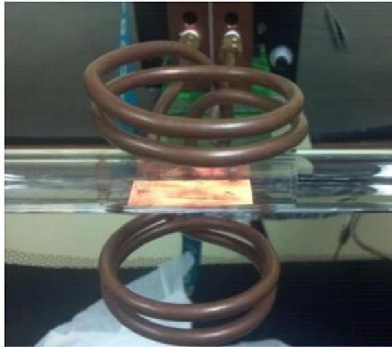
Figure 2.5. Photo of a 125  $\mu\text{m}$  thick 2 inch by 0.5 inch copper foil being heated by inductive heating.
