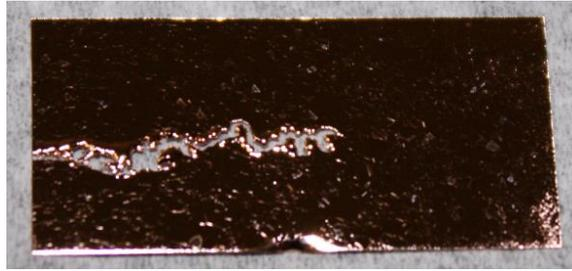
Figure 2.8. Photo of copper foil after localized melting in the inductively heated CVD system.
