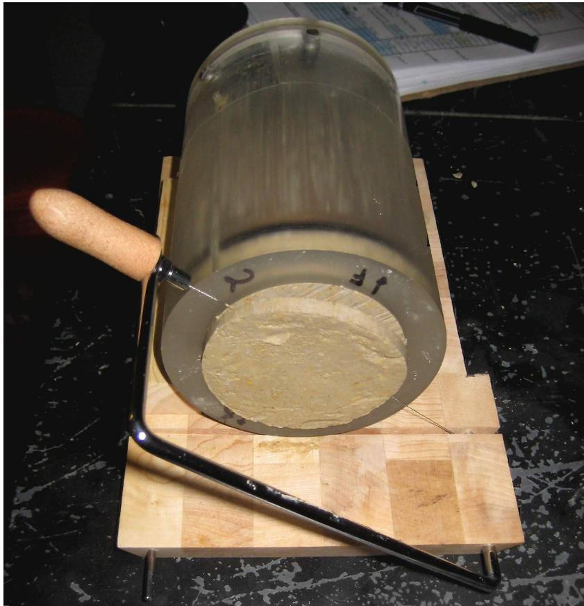
Figure 3.39: Trimming Centrifuge Test Specimen to Obtain the Water Content Profile
