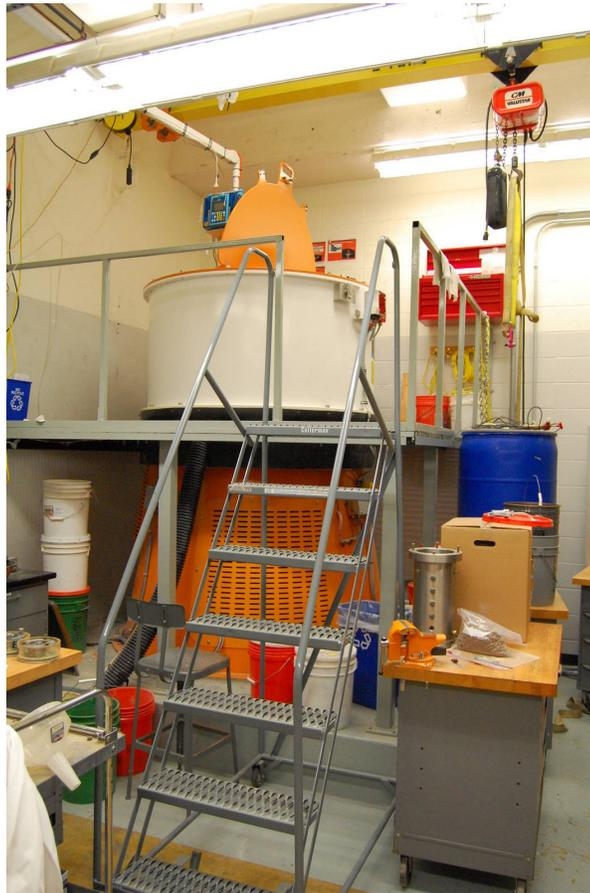
Figure 3.13: The Centrifuge Permeameter
