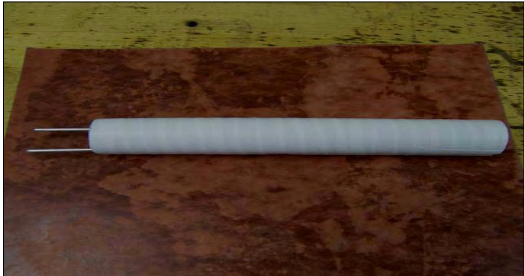
Figure 8.2: Step 2 of the preparation of propped fractures. Put the two halves of the core together with spacers between them and wrap them with a Teflon tape.
