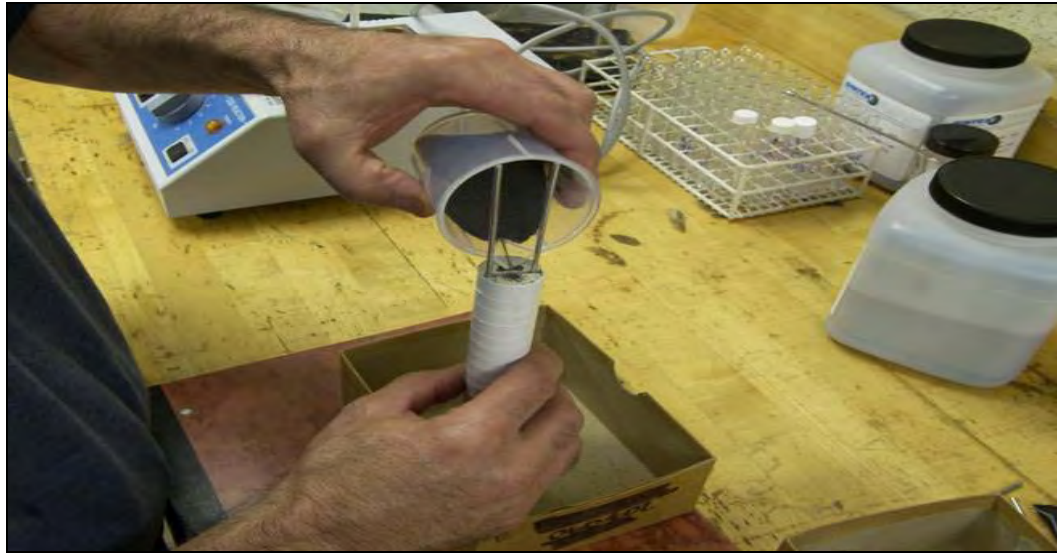
Figure 8.3: Step 3 of the preparation of propped fractures. Fill up the fracture space with proppant. Then wrap the core with a heat shrink tube.
