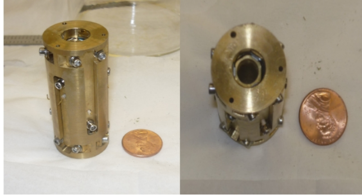
fig. 21: Completely assembled body of the STM.
