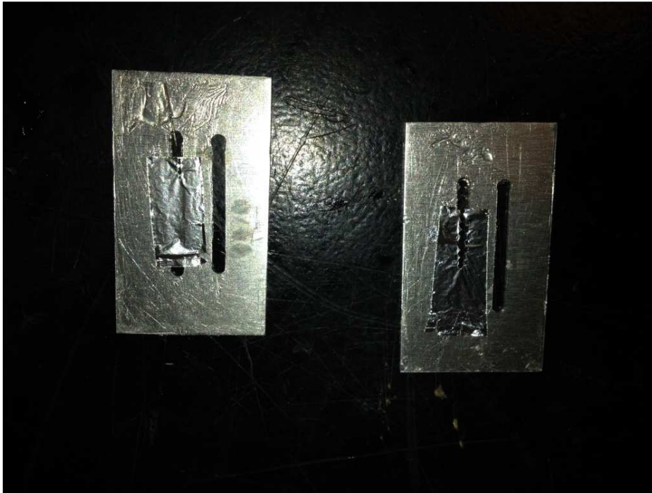
Figure 36: Typical image of 1.5 \mu m foils mounted on target holders. Foils were mounted on target holder with vacuum grease. The image on right shows the foil with holes from the laser.
