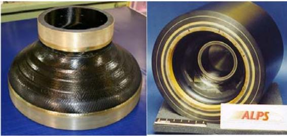
Figure 3. Composite arbor and dual arbor test rotor
