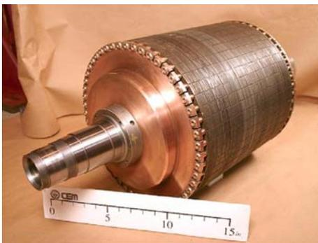
Figure 4. Rotor of high speed induction motor/generator
