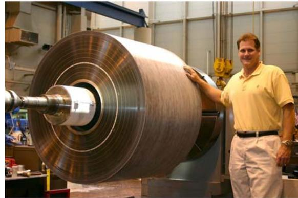
Figure 2. 480 MJ composite flywheel rotor
