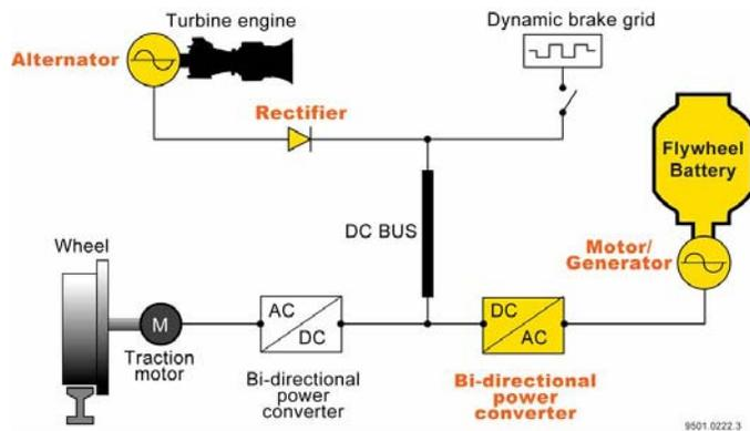
Figure 1. Simplified block diagram of ALPS system
