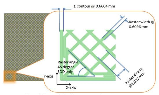
Figure 2: Sparse double dense cross section and parameters
