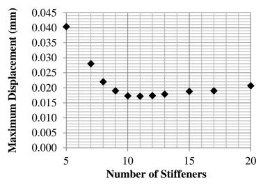
Figure 6: Maximum resultant displacement of TOI tools
