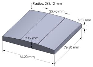
Figure 10: Verification tool geometry
