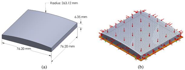
Figure 1: (a) Tool geometry and (b) loading condition
