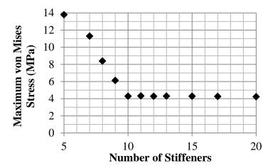
Figure 5: Maximum von Mises stress of TOI tools
