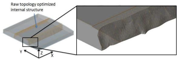
Figure 11: Topology optimization result for the verification tool
