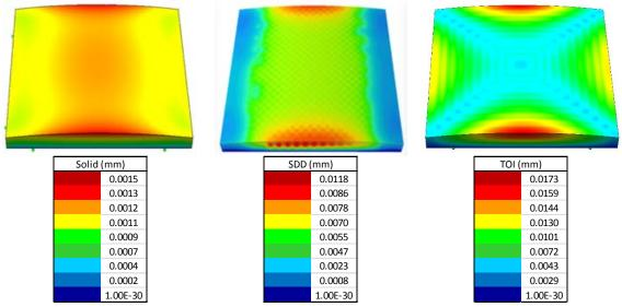
Figure 7: Resultant displacement contour plots
