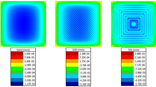
Figure 8: Z-axis displacement contour plots
