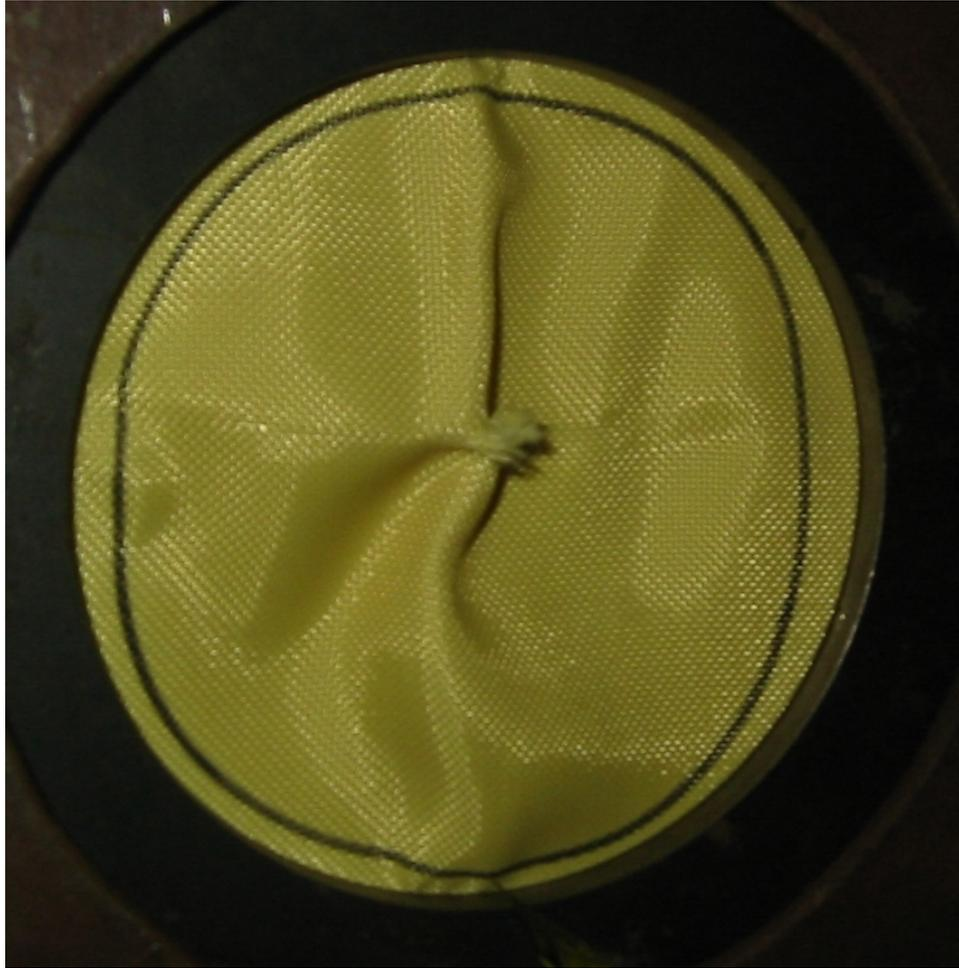
Figure 2.12: Post-impact damage for one layer of Kevlar with clamped edges
