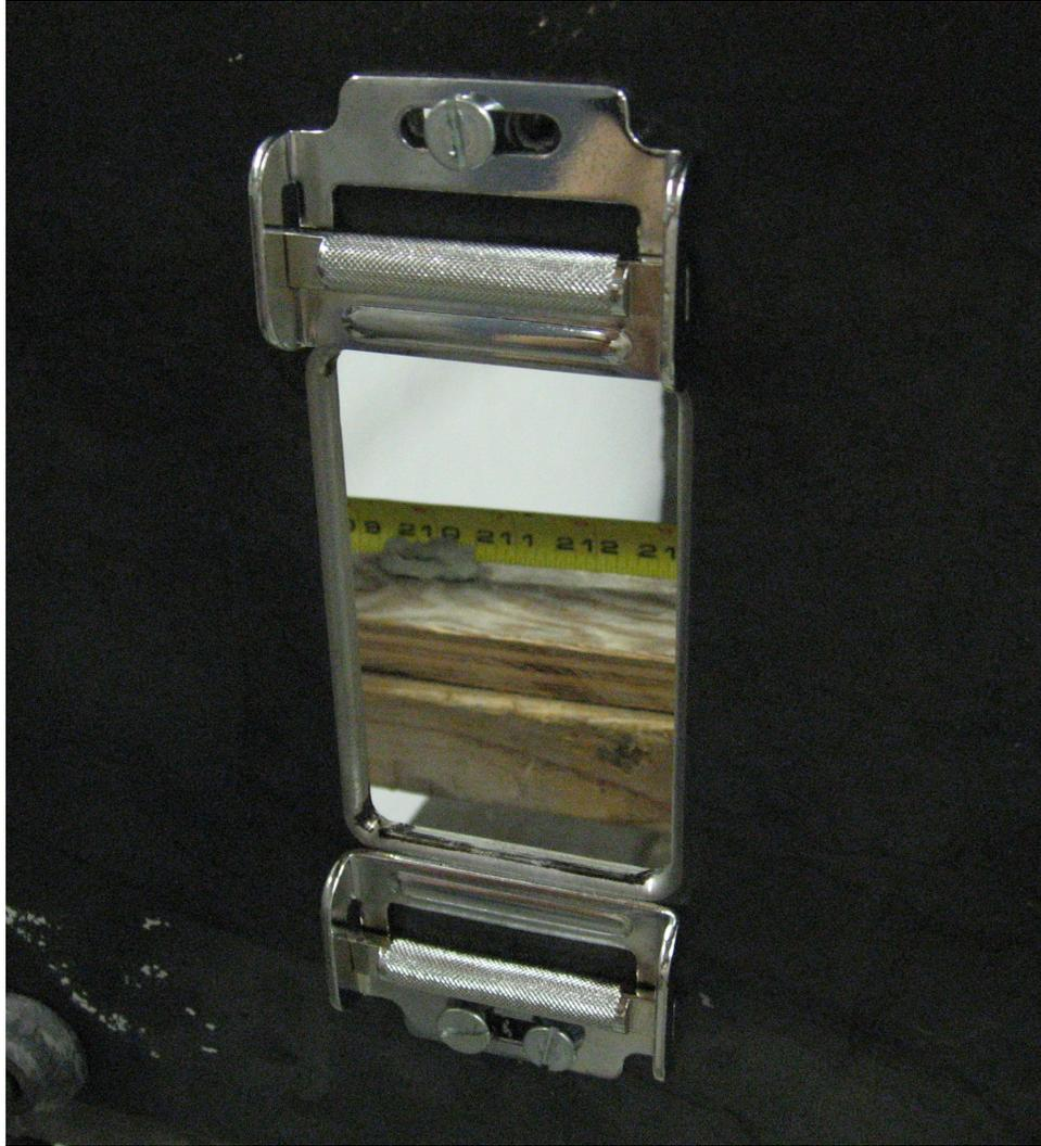
Figure 2.3: Cinch buckles for mounting the Kevlar in the two fixed and two free edges experiments
