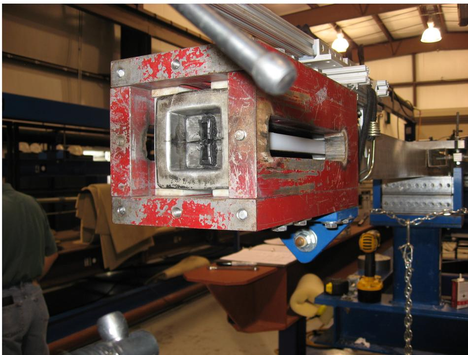
Figure 3.4: Sabot trap with a steel disk projectile sabot
