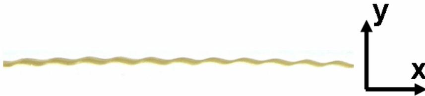
Figure 4.3: Crimp in Kevlar KM-2 yarn after removal from the woven fabric
