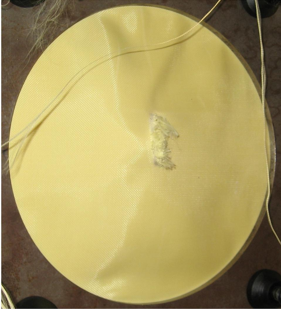
Figure 3.8: Post-impact damage by a steel disk projectile
