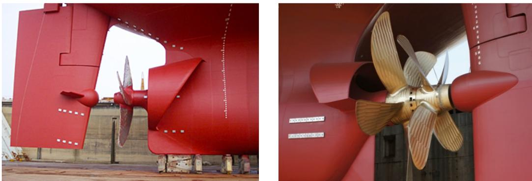
Figure 1.1: Side view of a ship stern (left) and counter-rotating propeller (right) (Source: [www.jmuc.co.jp](http://www.jmuc.co.jp) 05/02/2016).
