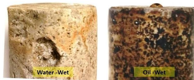
Figure 5.4: Silurian dolomite core before and after aging process
