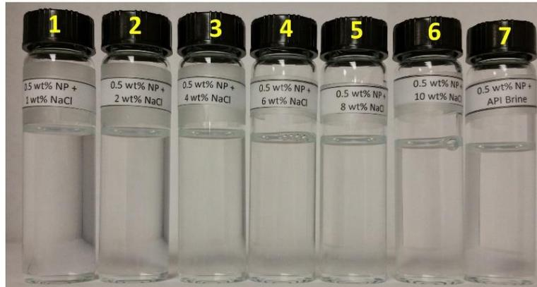
Figure 3.2: Samples containing 0.5 wt.% NP and 1, 2, 4, 6, 8, and 10 wt.% NaCl, and API brine (from left to right)
