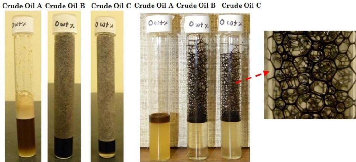
Figure 3.6: Foam morphology with 0.5 wt.% surfactant in the presence of oil at time (a)  $t=0$  minute (left); (b)  $t=8$  hr (right)
