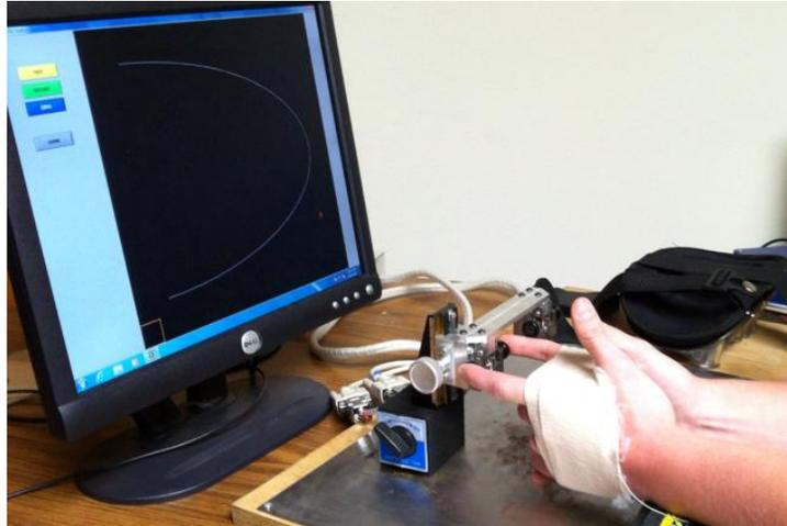
Figure 1- The manual force quantification system (MFQS) apparatus, including the monitor with target template and force transducers.
