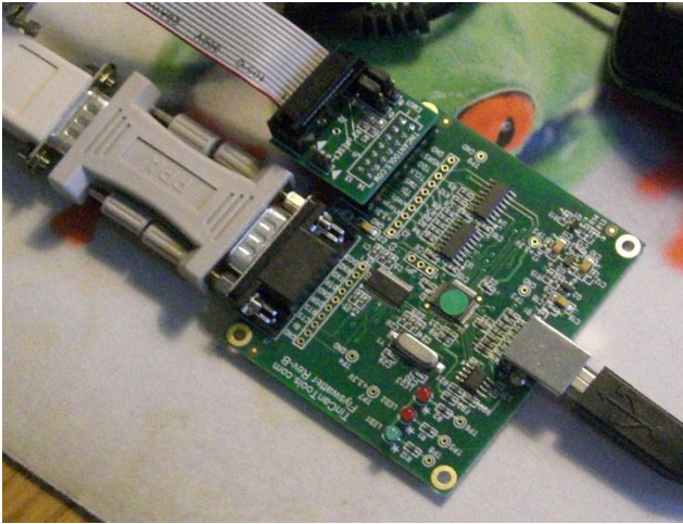
Illustration 3, FlySwatter in Circuit Debugger
