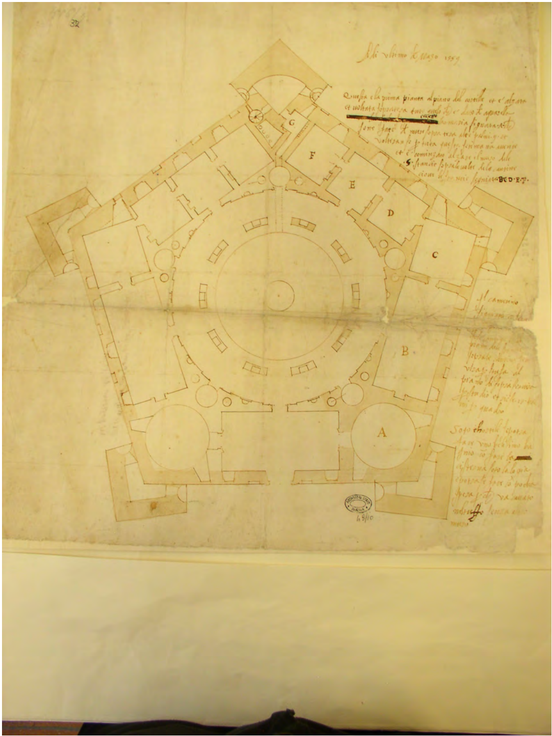
Fig. 6.43 Design drawing of the Villa Farnese at Caprarola by Vignola (ASP Piante e disegni 49 no.10, photo: author).
