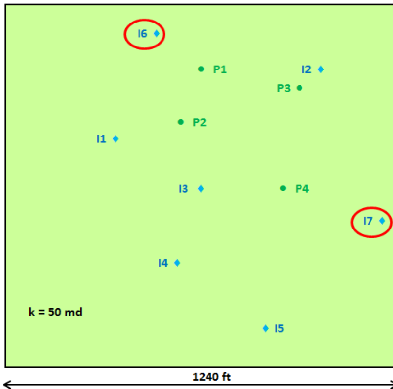
Figure 3.28: Synfield-5 is a homogeneous isotropic reservoir ( k=50 \text{ md} and \phi=0.2 ) and consists of five water injectors and four producers initially. After six years of oil production, two injectors (I6 and I7) have been added in the reservoir.
