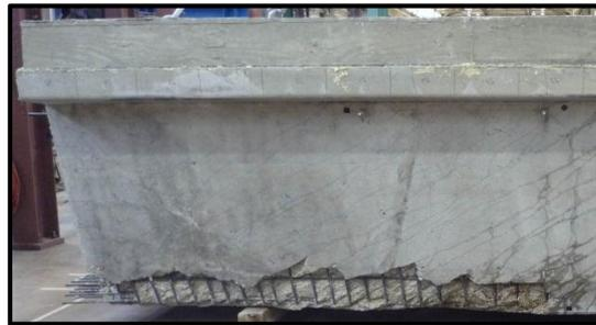
(B) Horizontal shear failure in Texas U54
