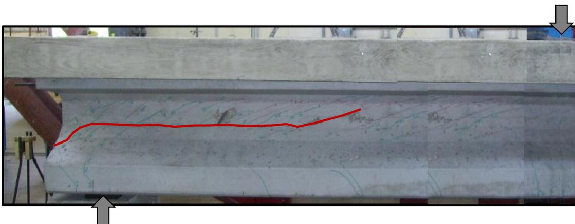
Figure 2-16: Tx28 after shear testing, with horizontal failure crack highlighted.
