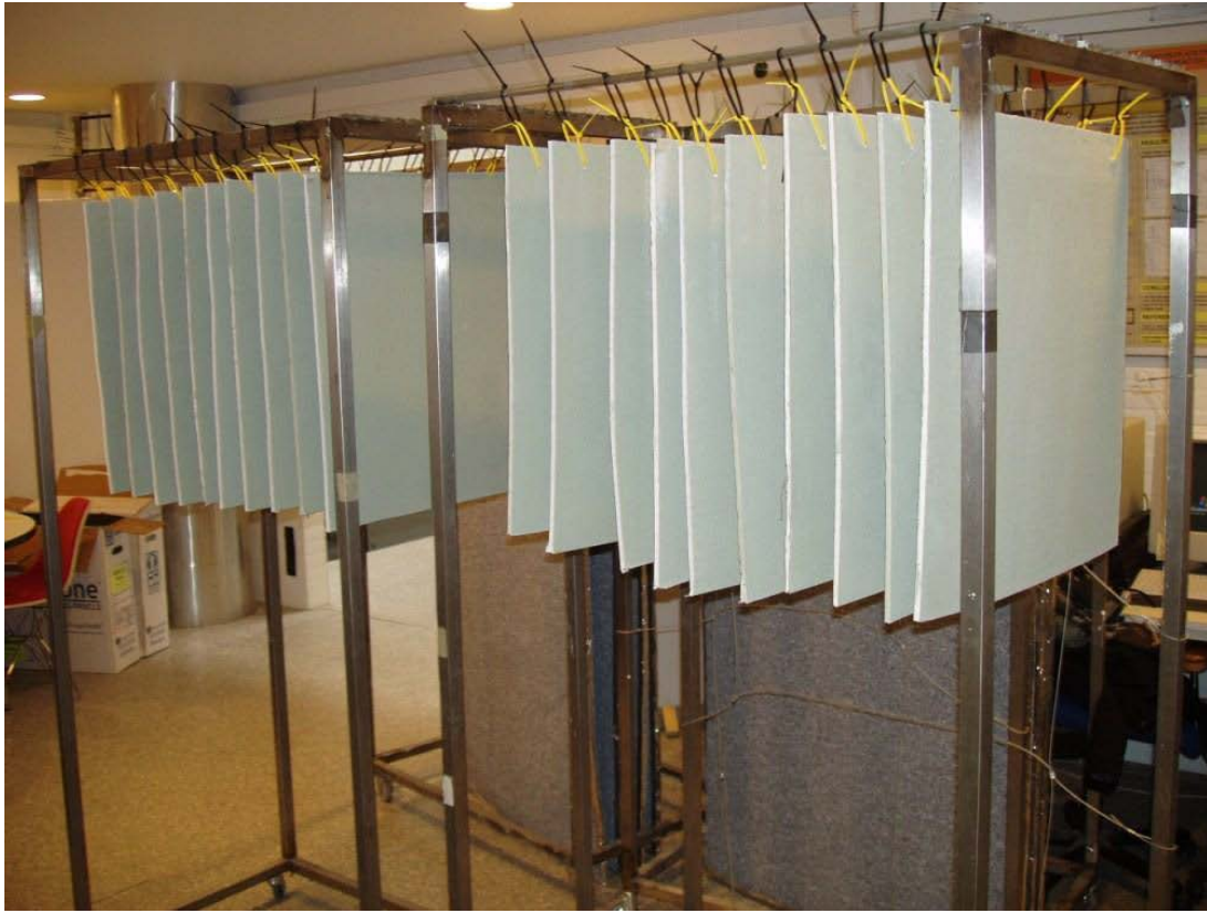
Figure F2: Configuration of clay plaster specimens on metal racks for PAQ analyses
