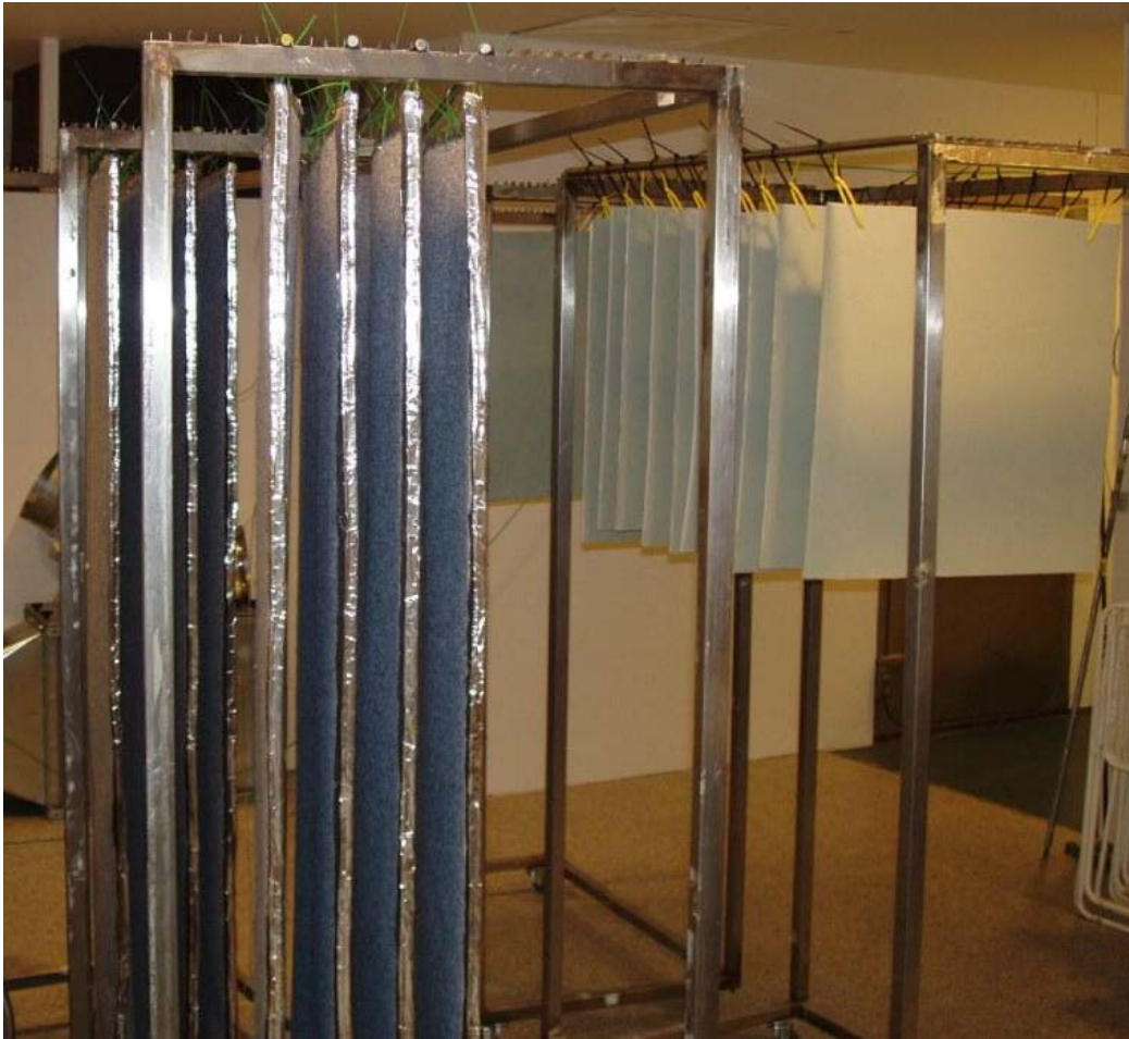
Figure F3: Configuration of carpet and clay plaster specimens on metal racks for PAQ analyses
