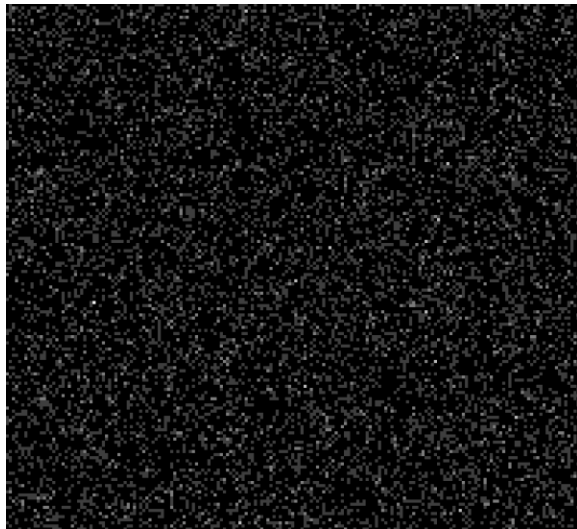
Figure 3.14: Background noise on a dark frame (contrast significantly increased to make noise more visible).
