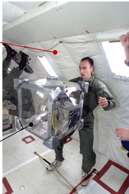
Figure 7.3: Image of author deploying a three degree-of-freedom attitude control experiment on a parabolic microgravity flight in April 2003. A similar experimental set-up could be used to test the SOAR Filter. The image on the right is jsc2003e27939 from [194], courtesy of NASA.
