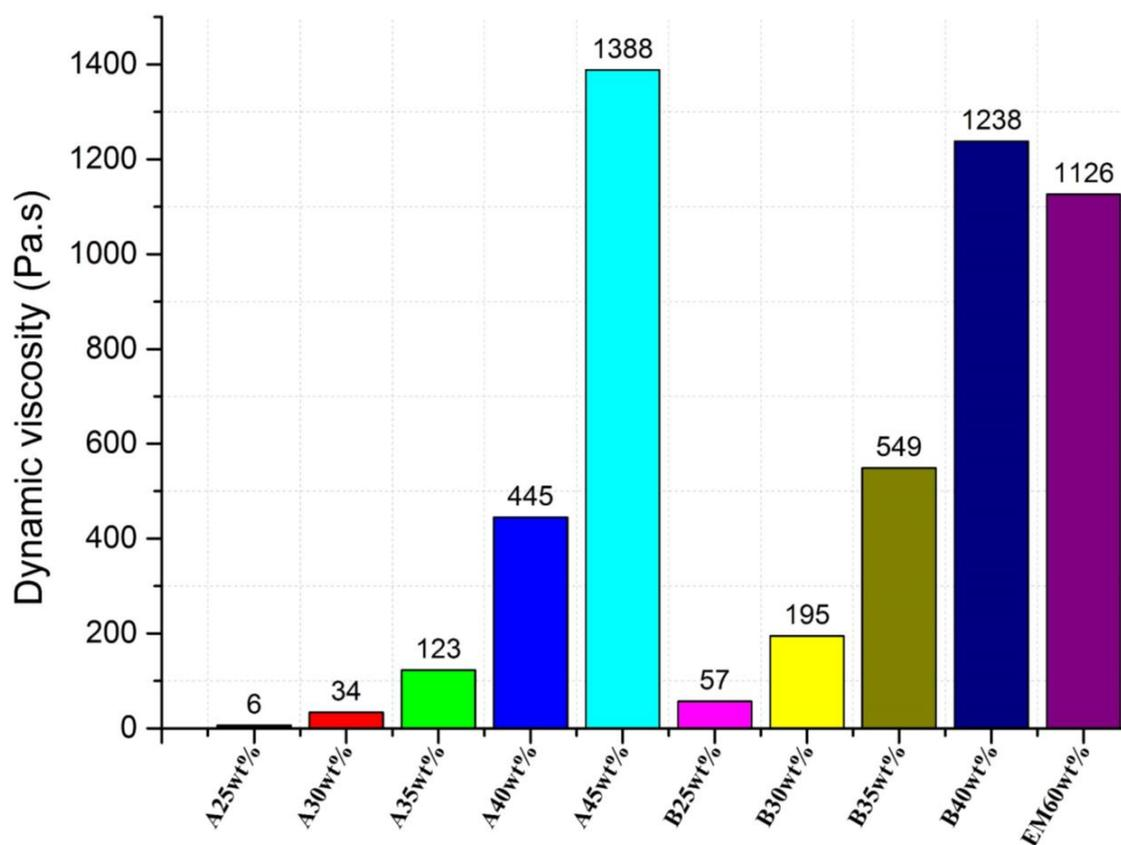
Figure 3 : Viscosity measurements of CA/acetone compositions
