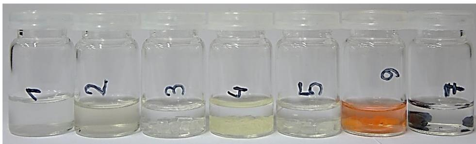
*Figure 1 : Solubility tests of inert materials in acetone. From left to right: EVA LEVAPREN® 700 HV (1); CA (2); EVAL™ (3); Rhodoviol 4/125 (4); Ultramid® 6A (5); PLA (6) and ABS (7)*
