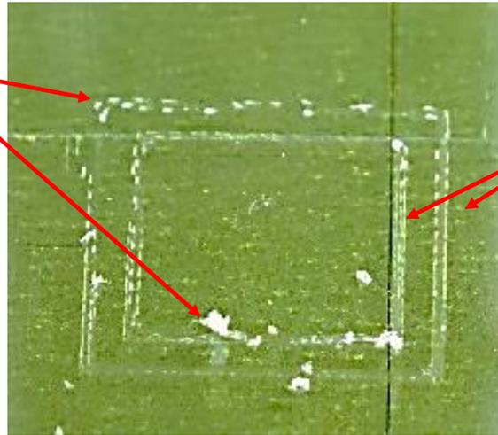
**Very good adhesion of the first deposited layer**
