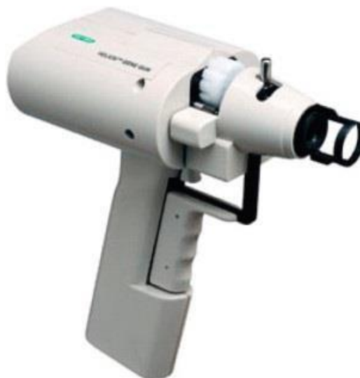
Figure 1.14: A Gene Gun. Gold nanoparticles are coated with the genetic vaccine and loaded onto a membrane. A compressed gas, such as helium, is used as the force that moved the filter down the barrel of the gun, which then pushes the membrane to a barrier. Once the membrane strikes the barrier, the force of the momentum will dislodge the nanoparticles from the membrane and they will travel beyond the barrel to interact with the target (cells, tissues, etc.). Figure from ref 249.
