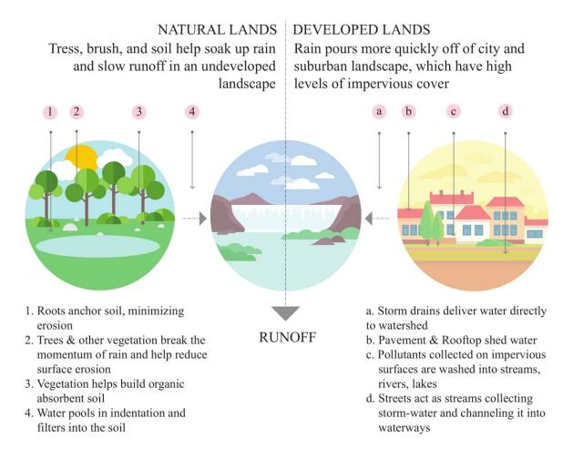
Figure 10 Impervious cover and urban drainage systems increase runoff to creeks and rivers. (Ruby, n.d.)
