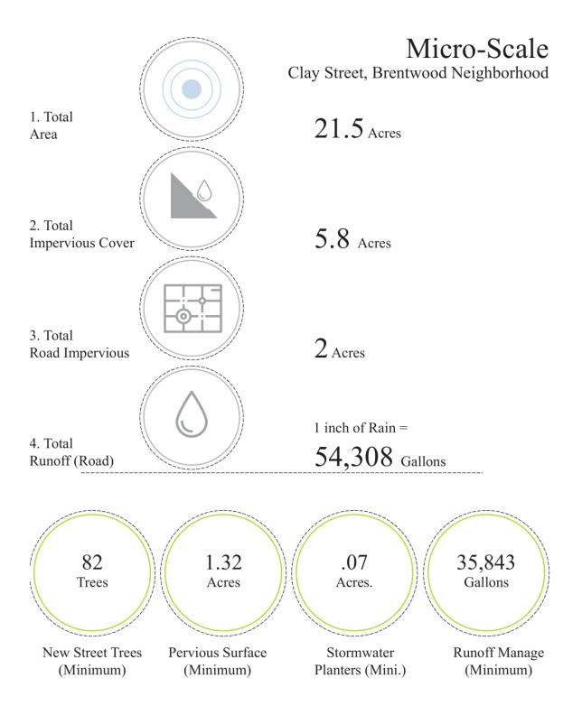
Figure 60 Calculation results for Clay Street
