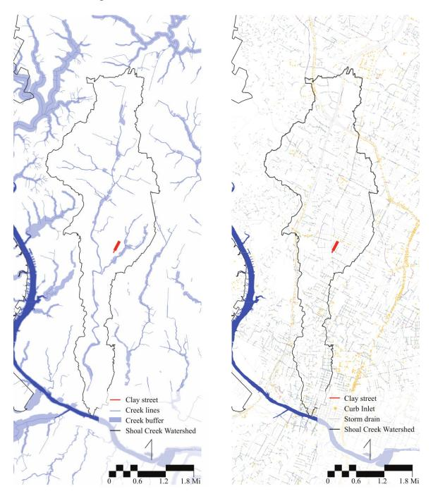
Figure 3 Shoal Creek Watershed- Natural stormwater system Vs. Man-made stormwater system.
