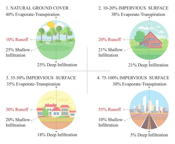
Figure 13Relationship between the impervious cover and surface runoff. ((EPA), n.d.)
