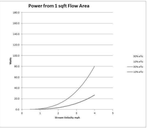
Figure 2.2. Power Potential from a Slow Flowing River
