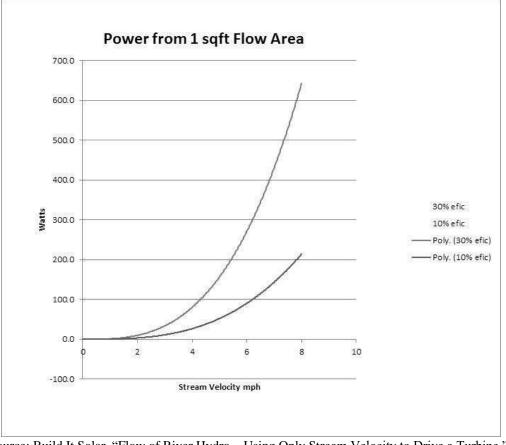
Figure 2.1. Power Potential from a Fast-Flowing River
