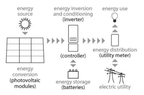
Figure 2.9. Solar Photovoltaic System Example
