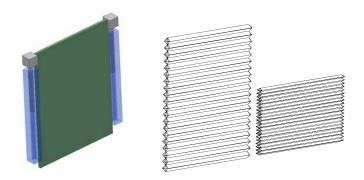
Figure 7: Trowel with adjustable length (left) and Expandable Trowel (right)
