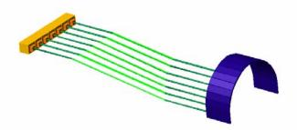
Figure 5: Trowels rotation to adjust for a curve output
