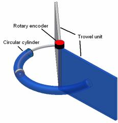
Figure 4: Trowel unit with circular cylinder
