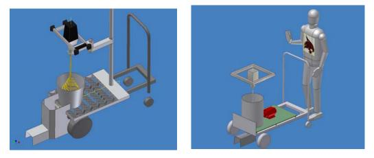
Figure 10: Design I: direct extrusion by centrifuge effect from mixer, Design II: direct extrusion by using vibrator and gravity effect
