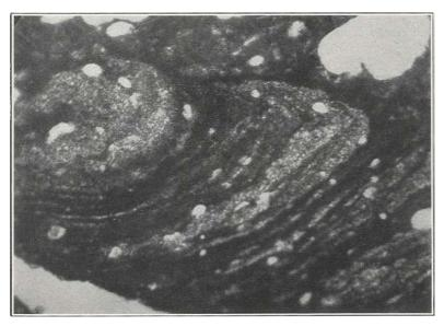
Fig. 2. Photomicrograph of fused shale showing flow structure.  $\times$  26.
