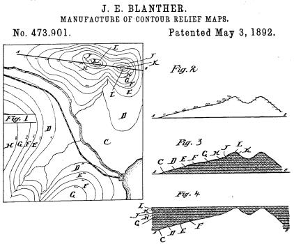
Figure 1: Blanther patent to fabricate 3-D relief map with layered method.
