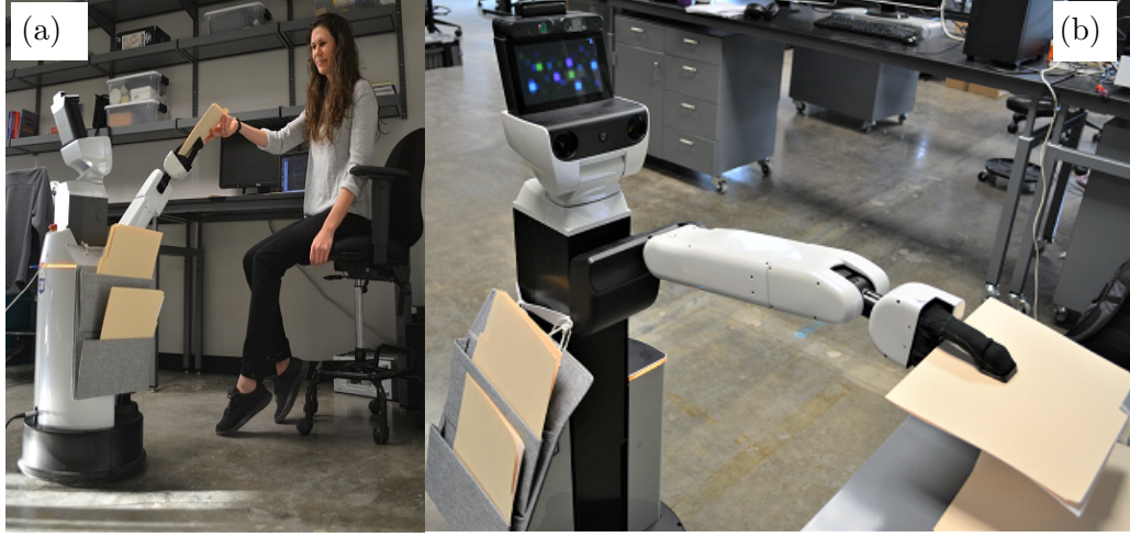
Figure 3.1: (a) The Toyota Human Support Robot, which we use as our experimental platform for human-informed work delivery, picking up completed work. (b) The HSR dropping off completed work at the Inventory Station.
