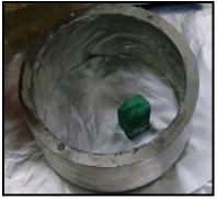
(a) Placing the lower half of the specimen ring on a sheet of aluminum and greasing the inner surface of the ring
