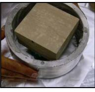
(b) Positioning the lower half of the specimen in the lower half of the ring
