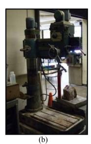
Figure 4.4: (a) Lapidary Slab Saw; (b) Core drill press
