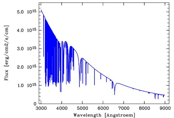
**Figure 1:** Model spectrum of a metal-polluted WD (GD 362). The large number of metal lines in the blue part contain Doppler information for the precise RV method. (model provided by D. Koester)
