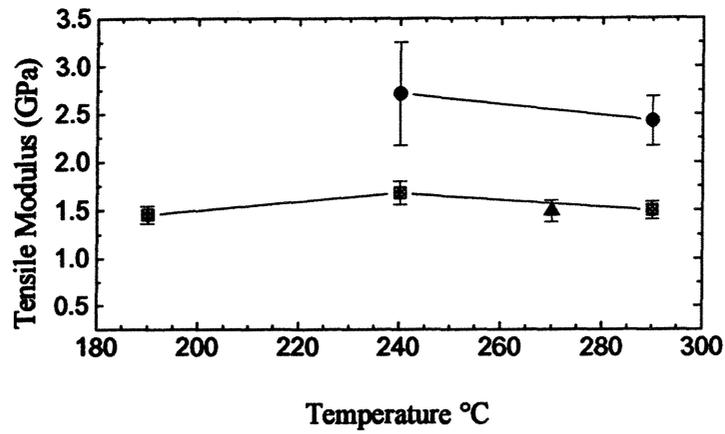
Figure 1 : Tensile modulus of Vectra A/PP (20/80 wt%) (—●—) and (40/60 wt%) (—■—) and ABS (—▲—) plaques built uniaxially in the machine direction as a function fabrication temperature.
