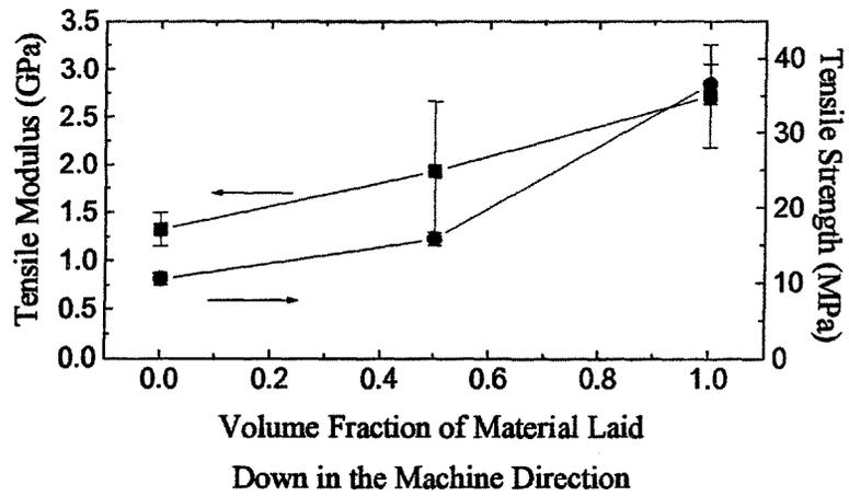
Figure 3: Tensile modulus (—■—) and strength (—●—) of Vectra A/PP (40/60 wt %) composite plaques fabricated via FDM as a function of volume fraction laid in the machine direction processed at 240°C.
