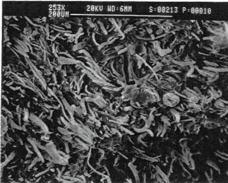
Figure 4 : Micrographs of the cross-section of Vectra A/PP (40/60 wt%) composite prototypes fabricated via FDM at 240°C.
