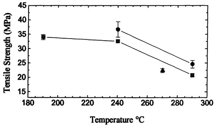
Figure 2 : Tensile strength of Vectra A/PP (20/80 wt%) (—●—) and (40/60 wt%) (—■—) and ABS (—▲—) plaques built uniaxially in the machine direction as a function fabrication temperature.
