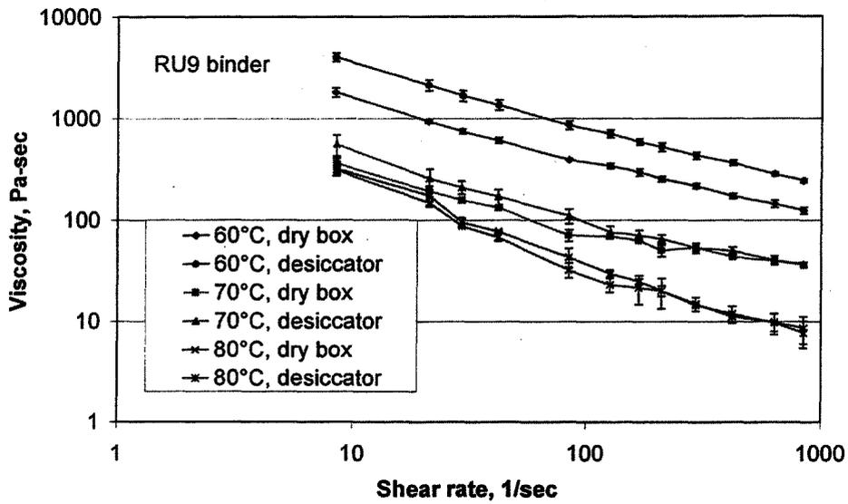
Figure 5. The viscosity vs. shear rate of RU9 binder stored in a dry box with 10% relative humidity and a desiccator with 100% relative humidity conditions, respectively, for 7 days.
