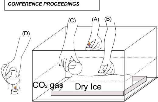
Figure 6. Testing for  $CO_2$  by extinguishing flame.
