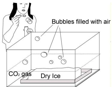
Figure 4. Using the property of density to test for  $CO_2$  gas that collects in the tank as the dry ice sublimes.
