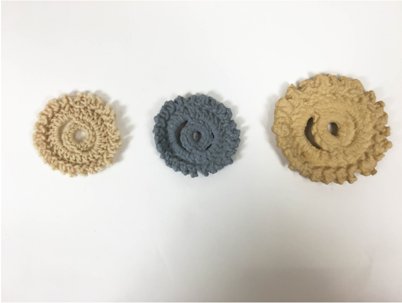
Figure 25. Dynamic pattern crocheted with acrylic yarn, 3D printed with PLA, and milled from MDF.
