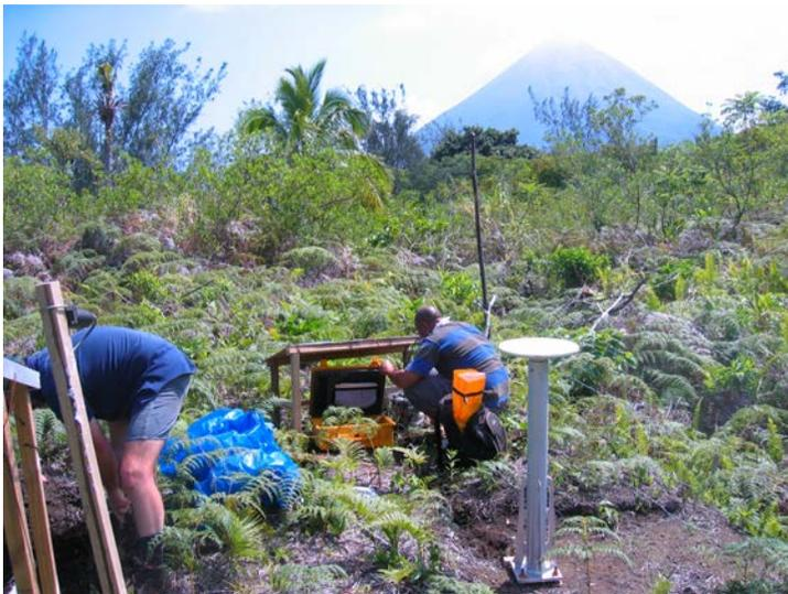
**Fig. 4. GPS station in the foreground at Tofua Island with Kao Island in the distance. A seismograph station was located just to the left. This GPS mast, bolted into a lava flow remains in place as do all of the others. They can be re-occupied at any time in the future to determine the net amount of motion that has occurred since October 2006 when we removed the instruments.**
