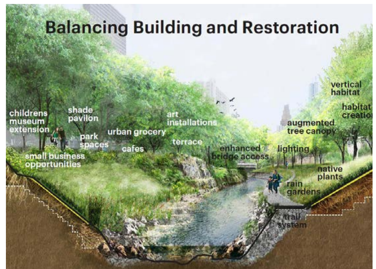
Figure 6. A cross section demonstrating the Waller District design approach, which includes instream habitat improvements, green stormwater methods, riparian restoration integrated with public access, and educational opportunities.
